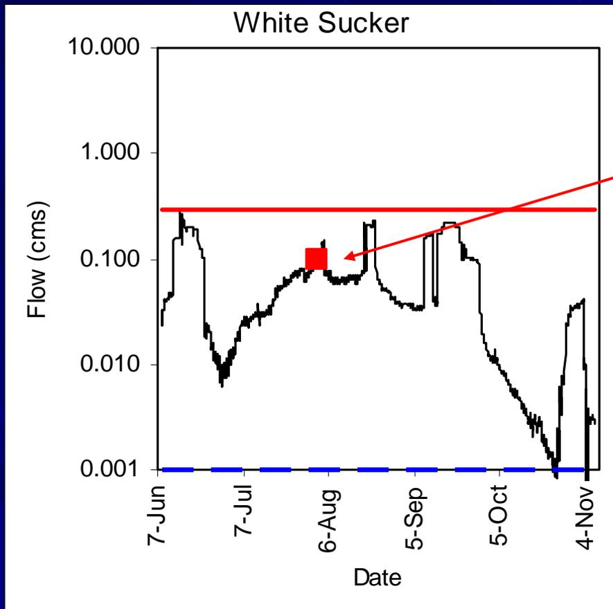
Passage window predicted by FishXing, but fish observed to not pass culvert, an example of case e)
