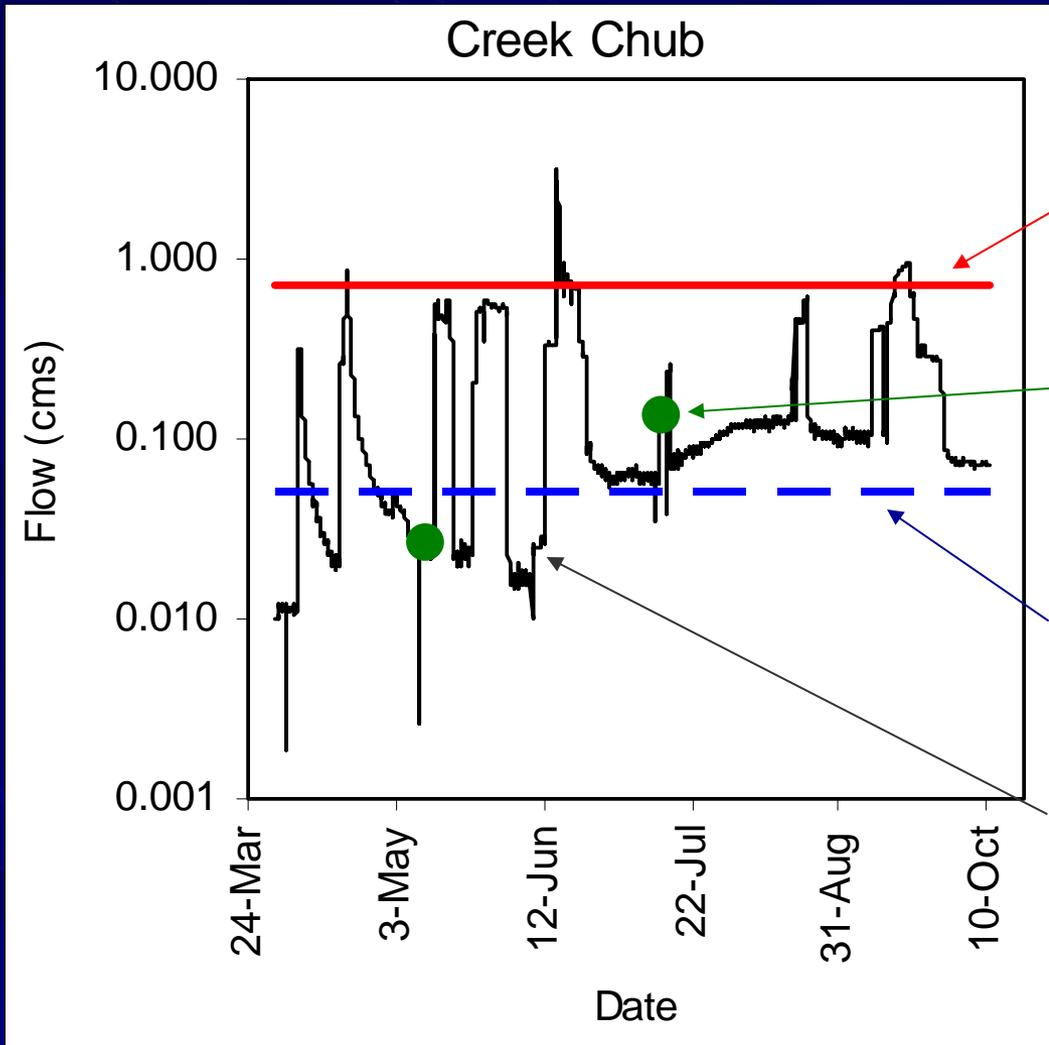
Highest flow where FishXing labels culvert non-barrier.
