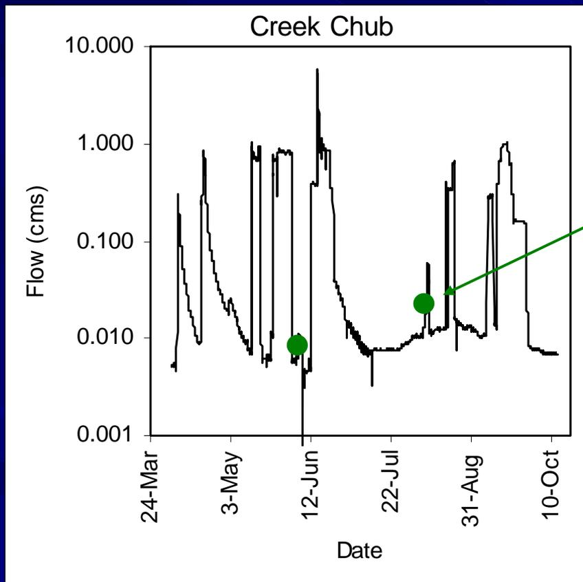
No passage window predicted by FishXing, and fish were observed to pass culvert.
