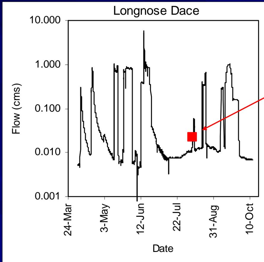
No window and fish observed to not pass culvert, an example of case c)
