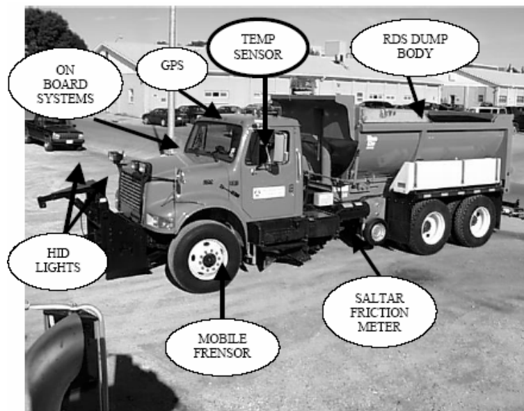
Figure 19. Highway maintenance concept vehicle and some of its components
