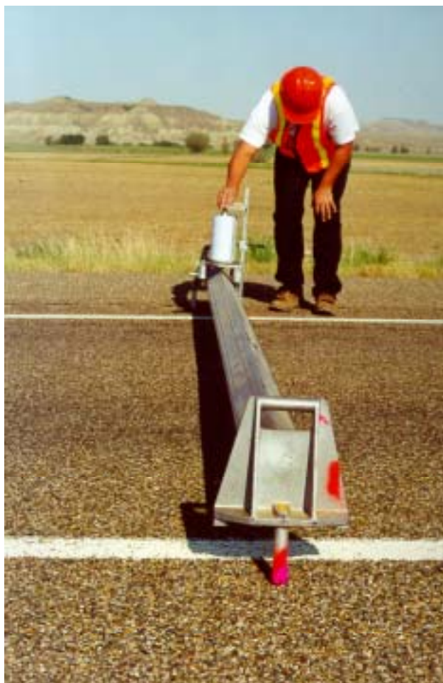
Figure 14. Moving the Rut-Transcribing Mechanism Across the Rainhart Profilograph
