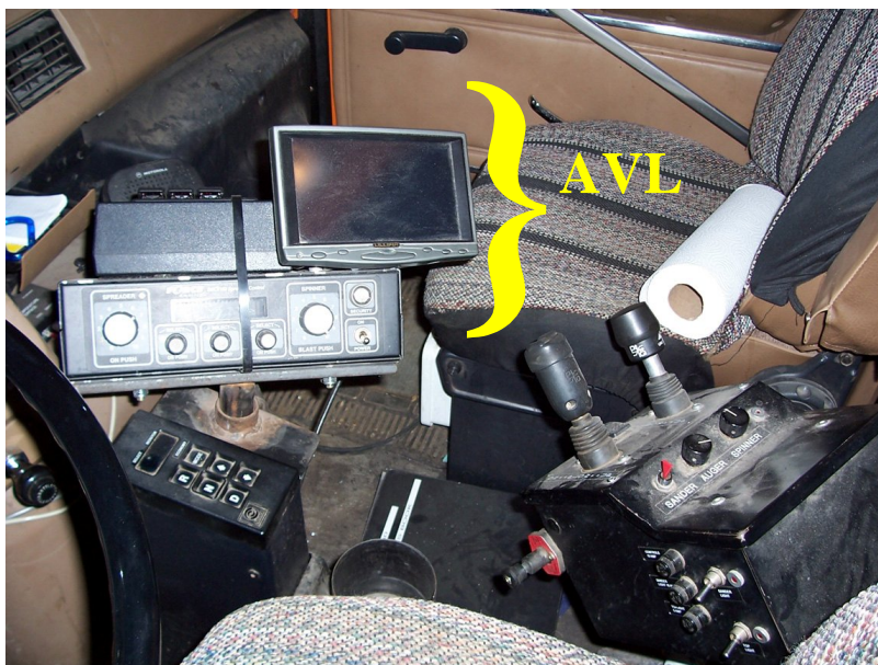
Figure 5-4: Helena Snowplow AVL In-Cab Equipment
