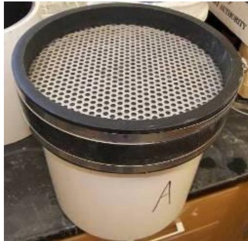
Figure 23. Support plate for bottom of specimen mold.
