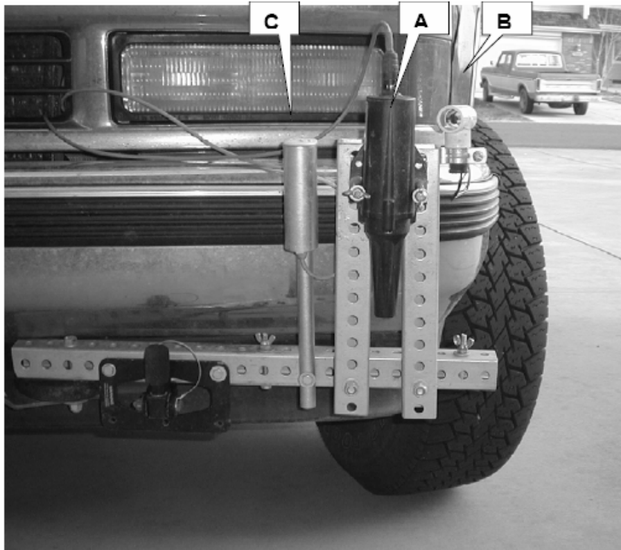
Figure 8: (A) Control Products IR Sensor, (B) Air Temperature Sensors, and (C) Roadwatch™ IR Sensor (from Tabler, 2004)
