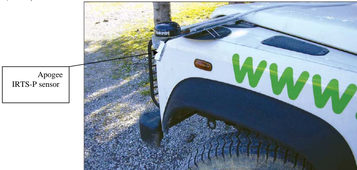
Figure 10: Apogee IRTS-P Sensor Installed on the Test Vehicle (from Campbell Scientific, Inc., 2004)
