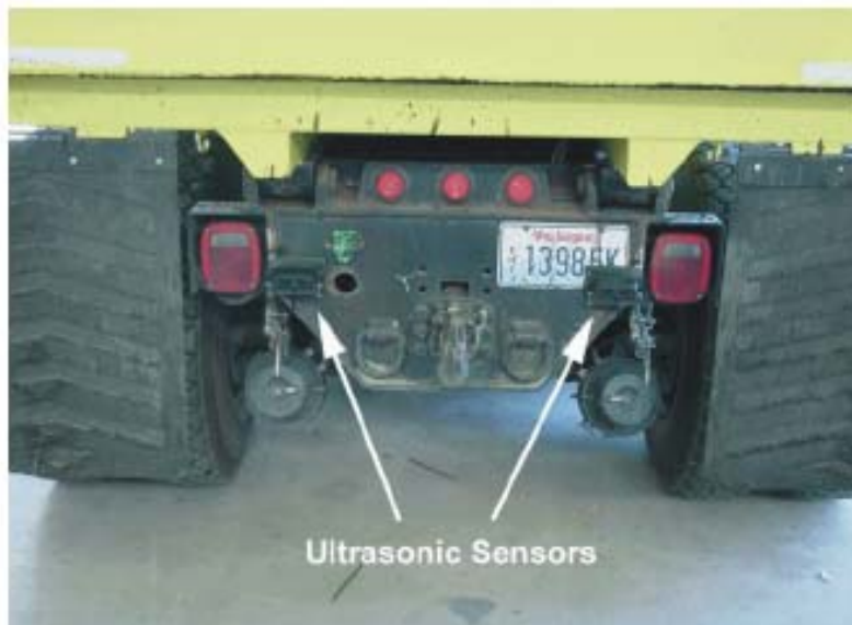
Figure 29: Hindsight Ultrasonic Sensor System (Graphic Courtesy of the National Institute for Occupational Safety and Health)
