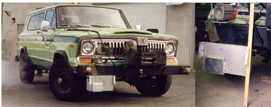
Figure 14: Sensor Mounted on CRREL Instrumented Research Vehicle (from Joshi, 2002)
