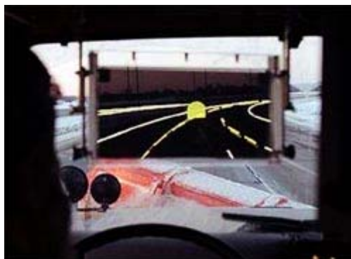
Figure 32: Driver's View through the HUD (from Lim et al., 2000)
