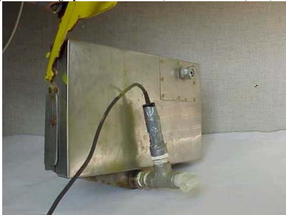
Figure 18: Photograph of Rear-View Collection Box with Conductivity Probe (from Garrick et al., 2002)
