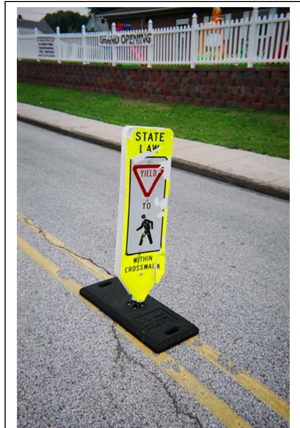
Figure 4-1: Example of YTPCD Damaged by Vehicle
