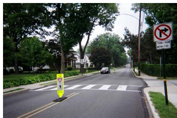
Figure 2-4: Example YTPCD Installation
