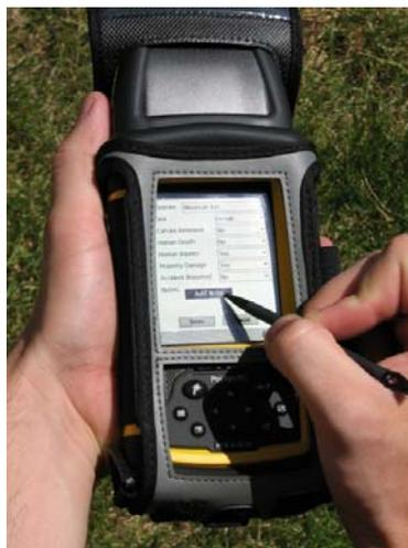
**Figure 3. PDA-GPS Hand-held Data Collector (Photo: Amanda Hardy/WTI).**
