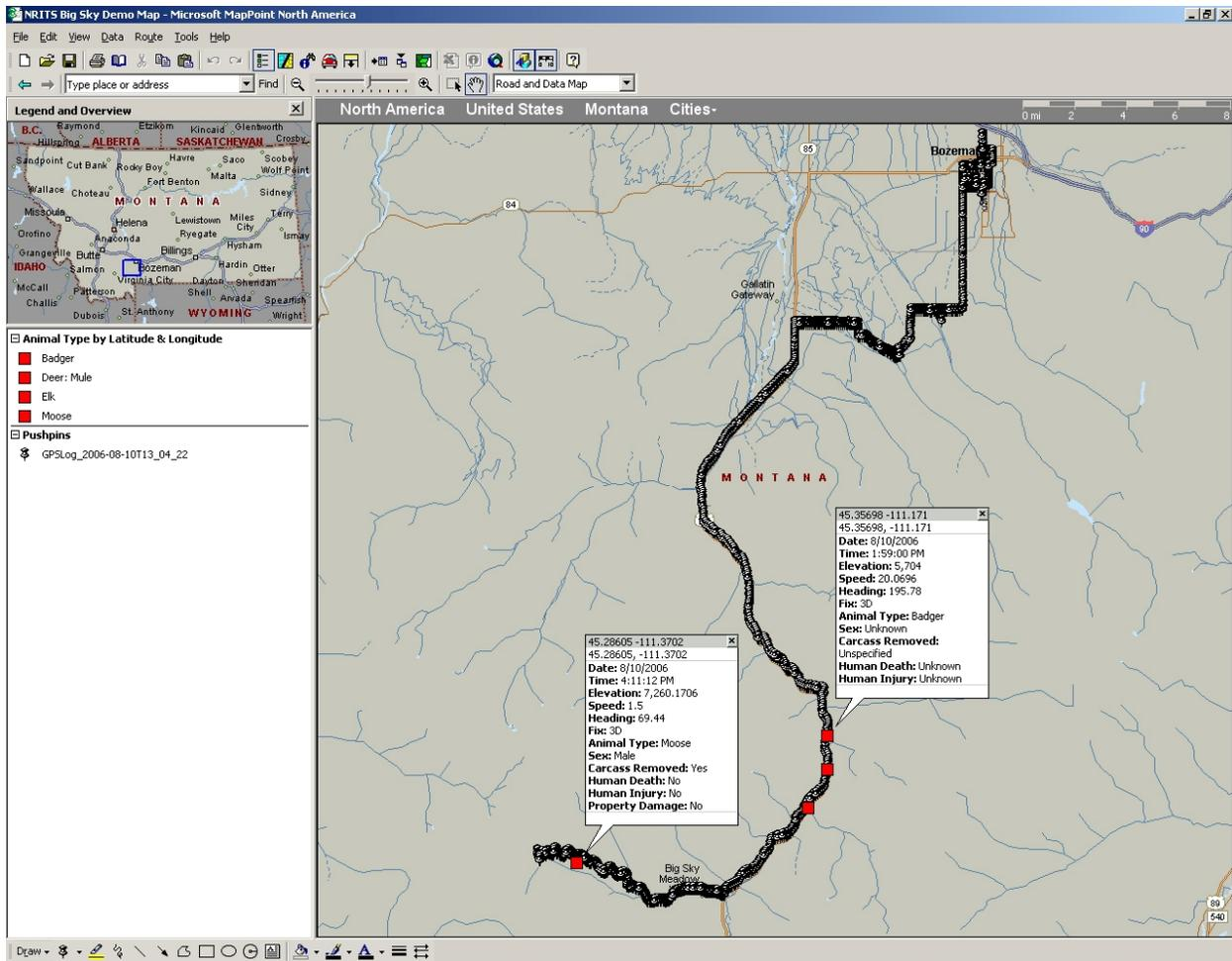
**Figure 4. Example of Output on a Map from an Approximate 45 mile Data Collection Session Along US Highway 191 in Montana with 4 Roadkills Recorded.**
