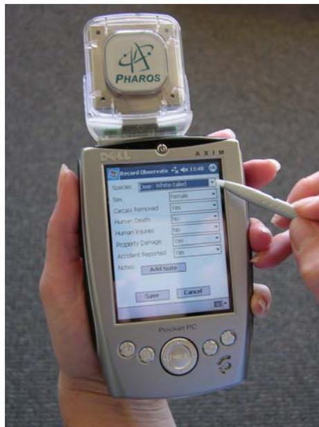
Figure 2. Proof-of-concept PDA-GPS hand held data collector (Photo: Marcel Huijser/WTI).
