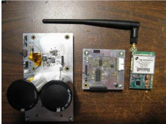
Figure 11. Voltage regulators and data collecting and transmitting system.
