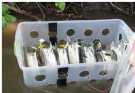
Figure 13. MFCs placed in the stream, featuring a simplistic enclosure.
