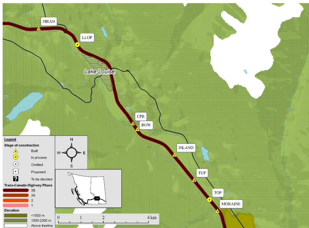
Figure 2.4: Phase IIIB-1 wildlife crossing structures on the Trans-Canada Highway (completion 2009).
