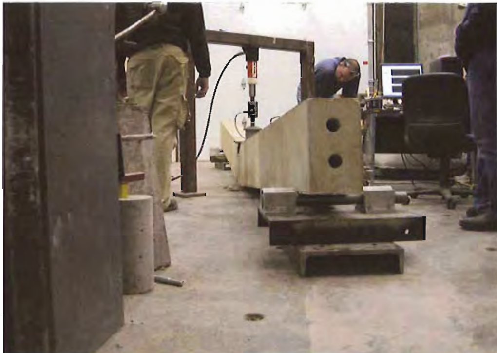
Half scale beam test at failure. (November 2007) Kyle Applebury is inspecting the flexural cracks.
