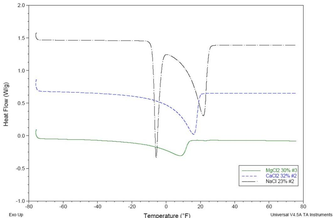
**Figure 8: DSC thermograms of 23% NaCl, 32%  $\text{CaCl}_2$ , and 30%  $\text{MgCl}_2$ , dilution 3:1, warming cycle,  $3.6^\circ\text{F}/\text{minute}$**
