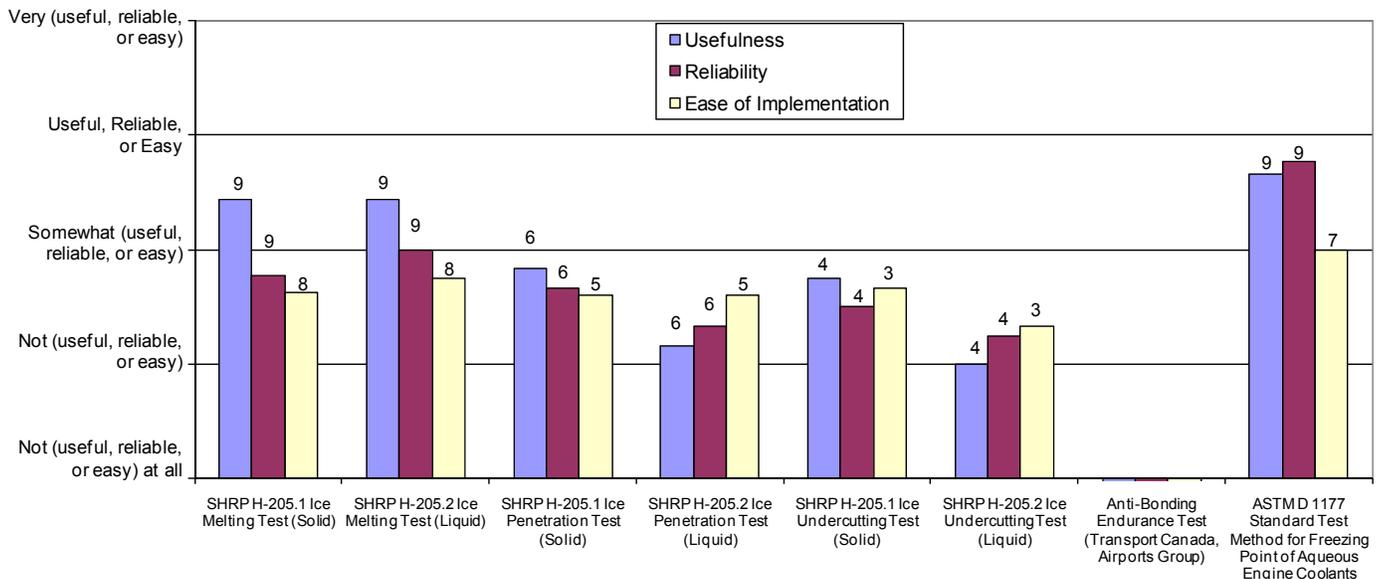
**Figure 3: The average ranking for usefulness, reliability, and ease of implementation of various deicer performance tests, with number of responses shown above each bar**
