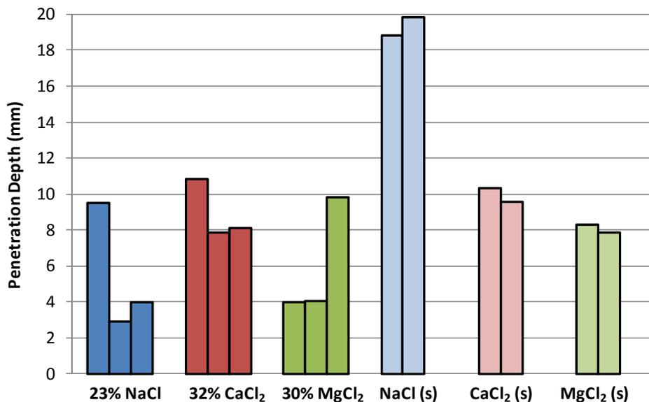
**Figure 14: Modified SHRP Ice Penetration Test results at 60 minutes at  $30^\circ\text{F}$**
