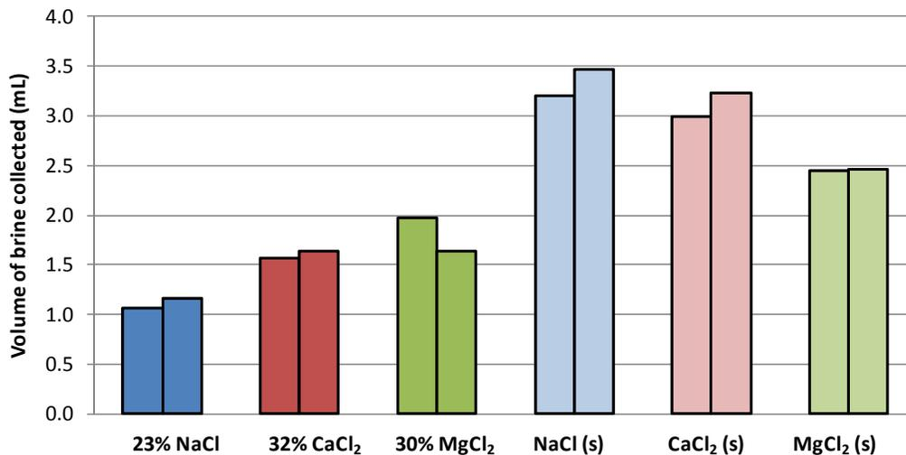
**Figure 12: Modified SHRP Ice Melting Test results at 60 minutes at 15°F**
