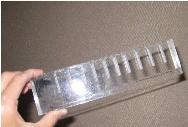
Figure 13: SHRP Ice Penetration Test apparatus
