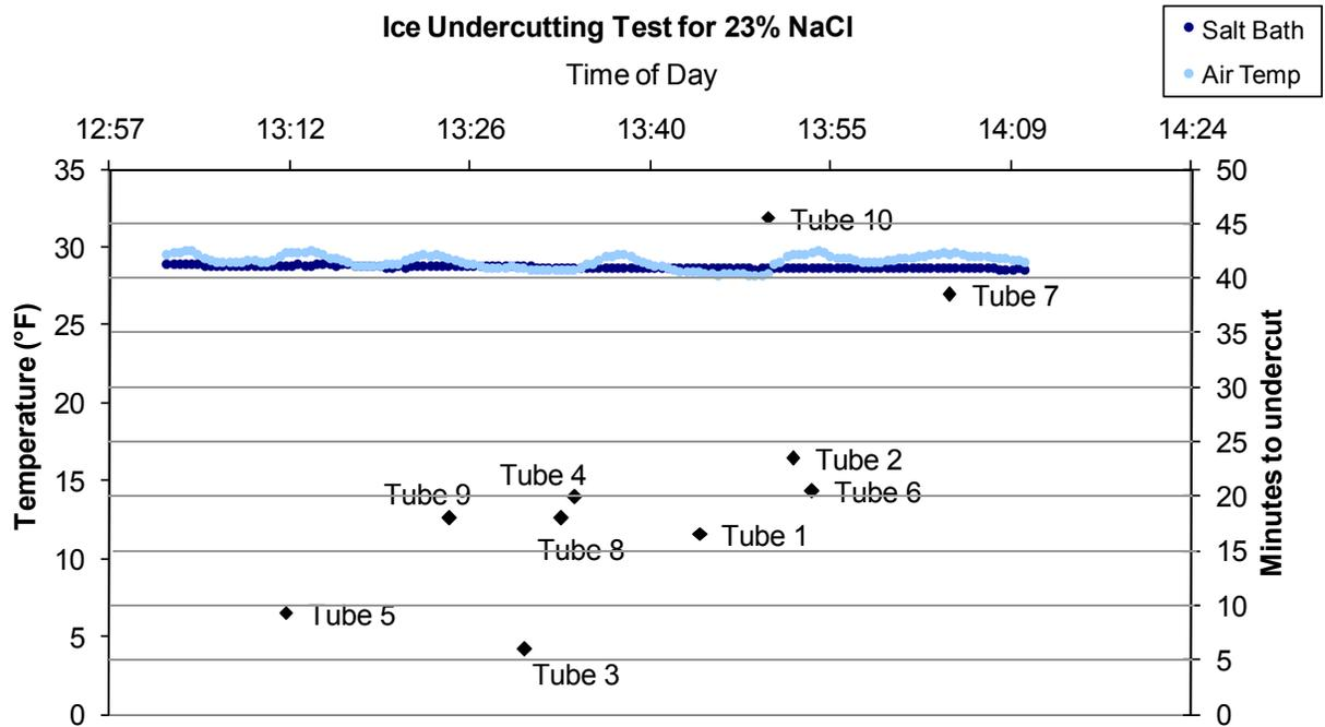
Figure 16: Sample result for ice undercutting test using 23% NaCl at 30°F
