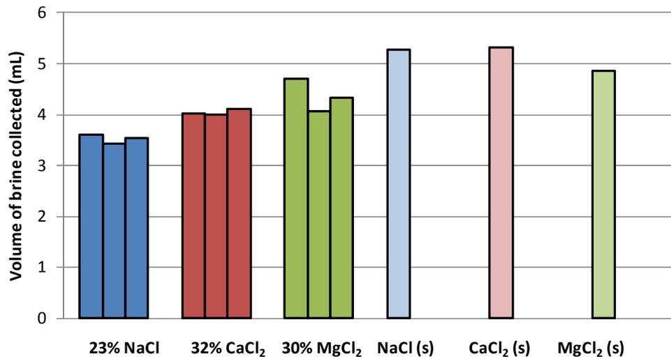
**Figure 11: Modified SHRP Ice Melting Test results at 60 minutes at 30°F**
