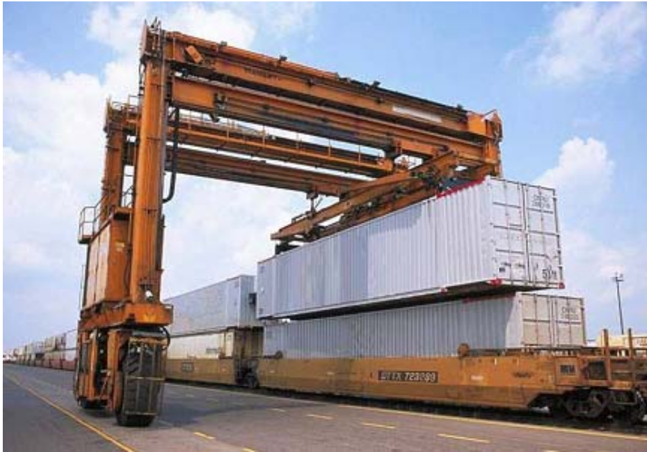
Figure 7: Top-Load, Top-Pick Gantry (CH2M Hill 2008).
