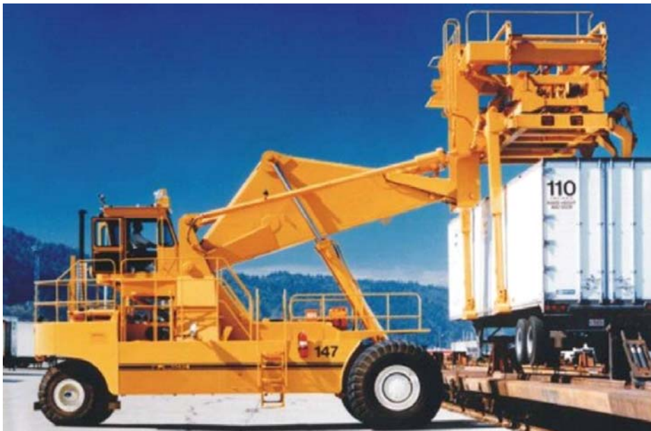
Figure 6: Side-load, Bottom-pick Loader (CH2M Hill 2008).
