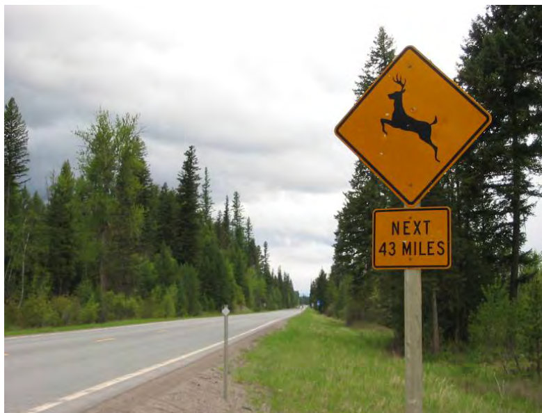
Figure 7: Standard deer warning sign on Highway 83 in Montana includes the length of the road section that the warning sign applies to (© Marcel Huijser).
