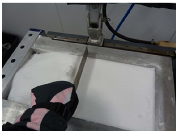
Figure 7: Grated snow is sieved onto the pavement sample (left) and leveled with a screed (right).
