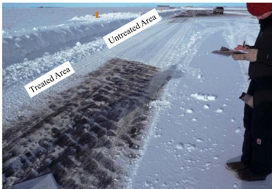
Figure 45: Treated and untreated areas of special asphalt section (MgCl).
