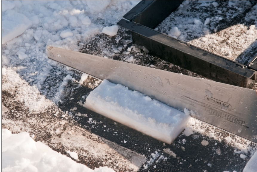
Figure 48: Cutting a snow sample for bond strength testing.
