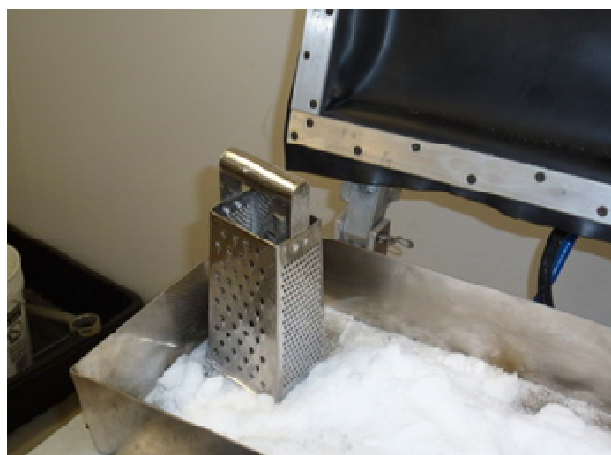
Figure 7: Grated snow is sieved onto the pavement sample (left) and leveled with a screed (right).
