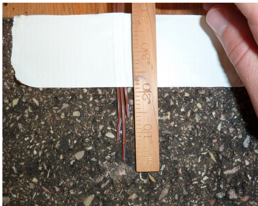
Figure 22: Positioning of thermocouples under the snow sample.
