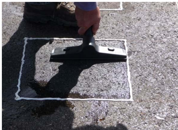
FIGURE 36 Sample collection using a vacuum with squeegee attachment.
