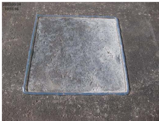
Figure 33 Evidence of the applied liquid deicer NaCl+GLT remains in the test box
