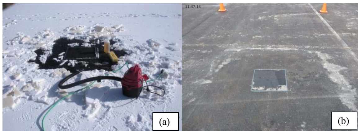
Figure 31 Sample test box shown after melting snow accumulation, replacement, agitation, and vacuum sample collection (a) and a test section with no snow and deicer visible in the unsampled test plot (b).
