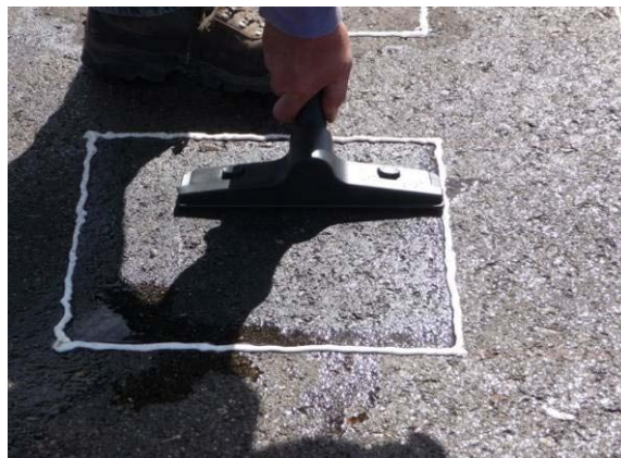
Figure 16 Sample collection using a vacuum with squeegee attachment.
