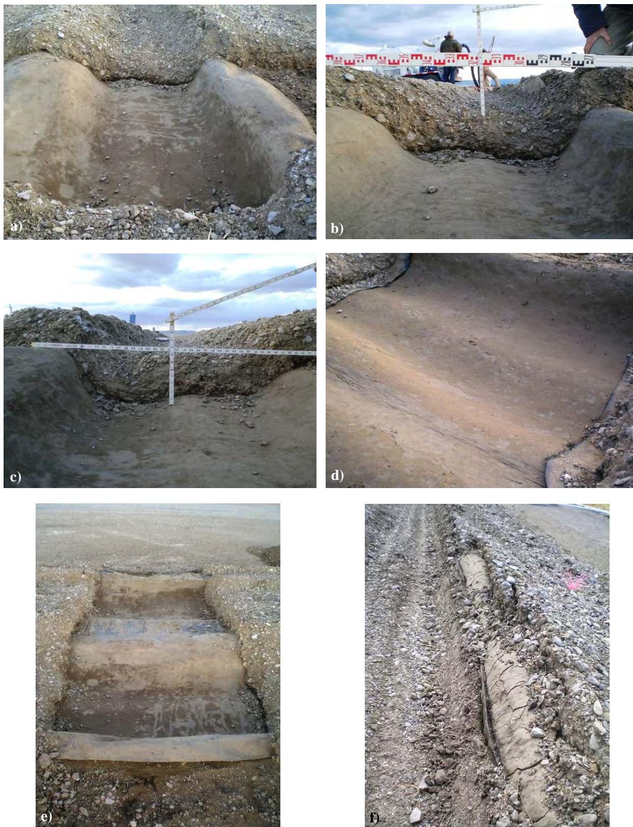
Figure C-31. Photos of the forensic excavations of the WoT-9 test section: a) rut bowl, b) base rut profile, c) subgrade rut profile, d) subgrade surface, e) looking east and f) pullout failure.
