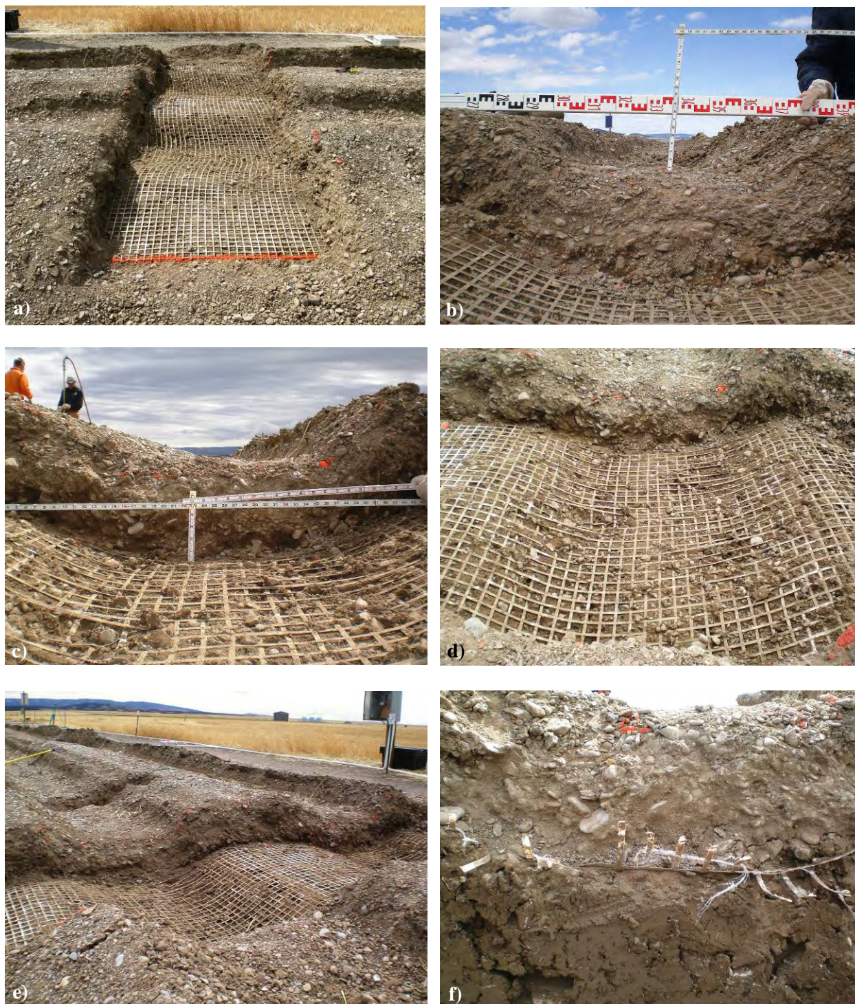
Figure C-22. Photos of the forensic excavations of the WeG-6 test section: a) looking west, b) base rut profile, c) subgrade rut profile, d) rut bowl, e) view from the side and f) layering of base and subgrade.
