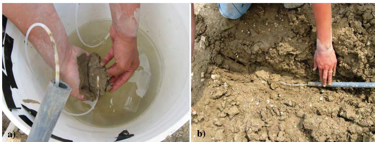
Figure 10. Installation of pore water pressure sensors: a) encapsulating porous stone with saturated subgrade, b) burying in subgrade.
