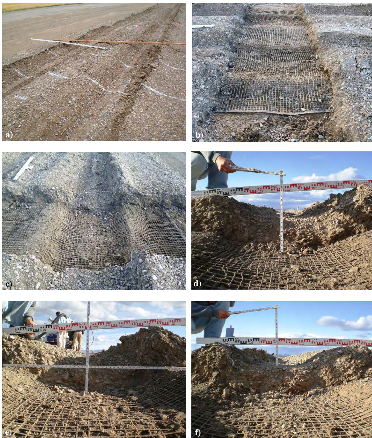
Figure C-25. Photos of the forensic excavations of the WoG-7 test section: a) excavation area, b) looking west, c) rut bowl, d) subgrade rut profile, e) subgrade rut profile and f) base rut profile.
