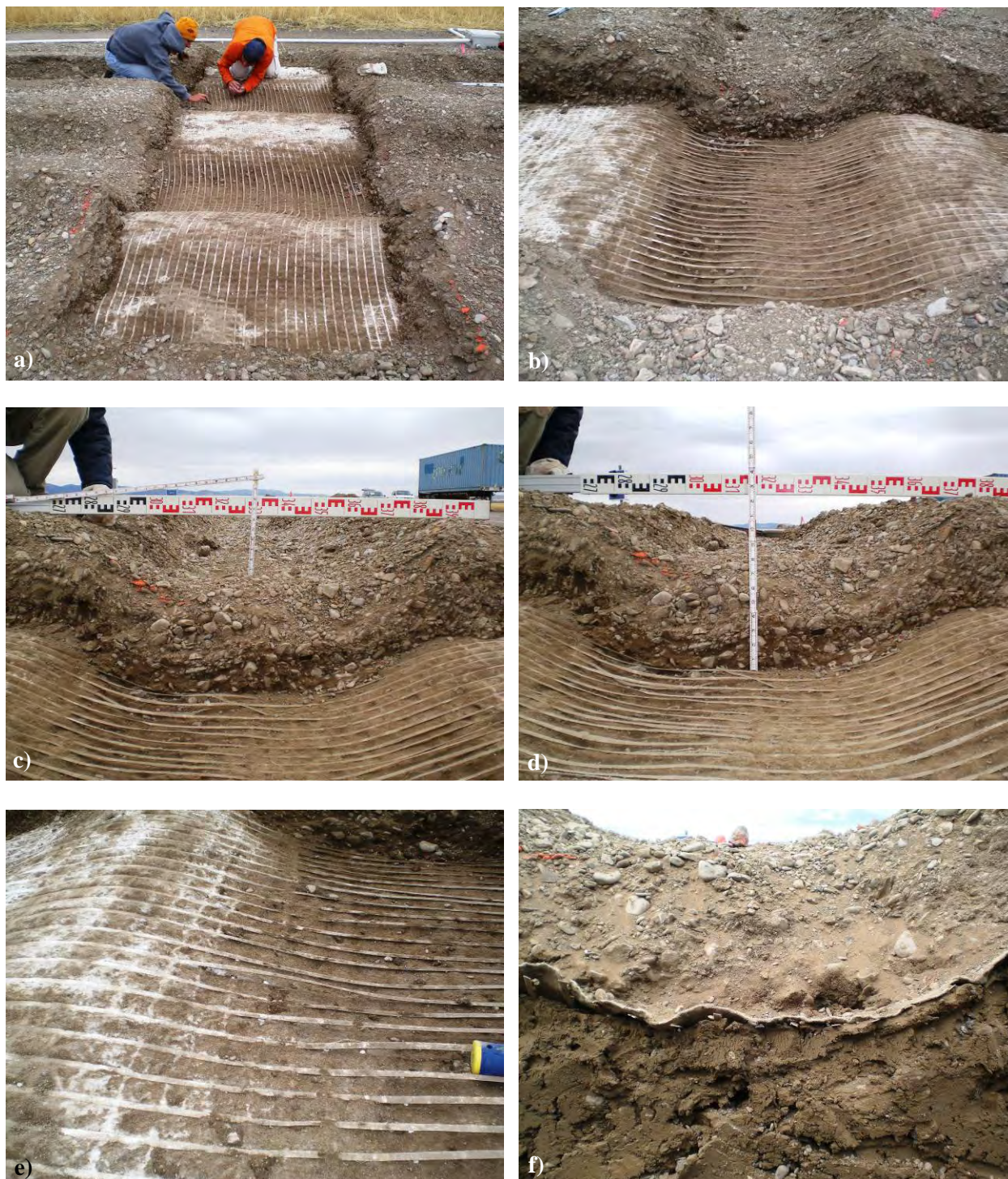
Figure C-17. Photos of the forensic excavations of the CoG-4 test section: a) looking west, b) rut bowl, c) base rut profile, d) subgrade rut profile, e) close-up of rut and f) layering of base and subgrade.
