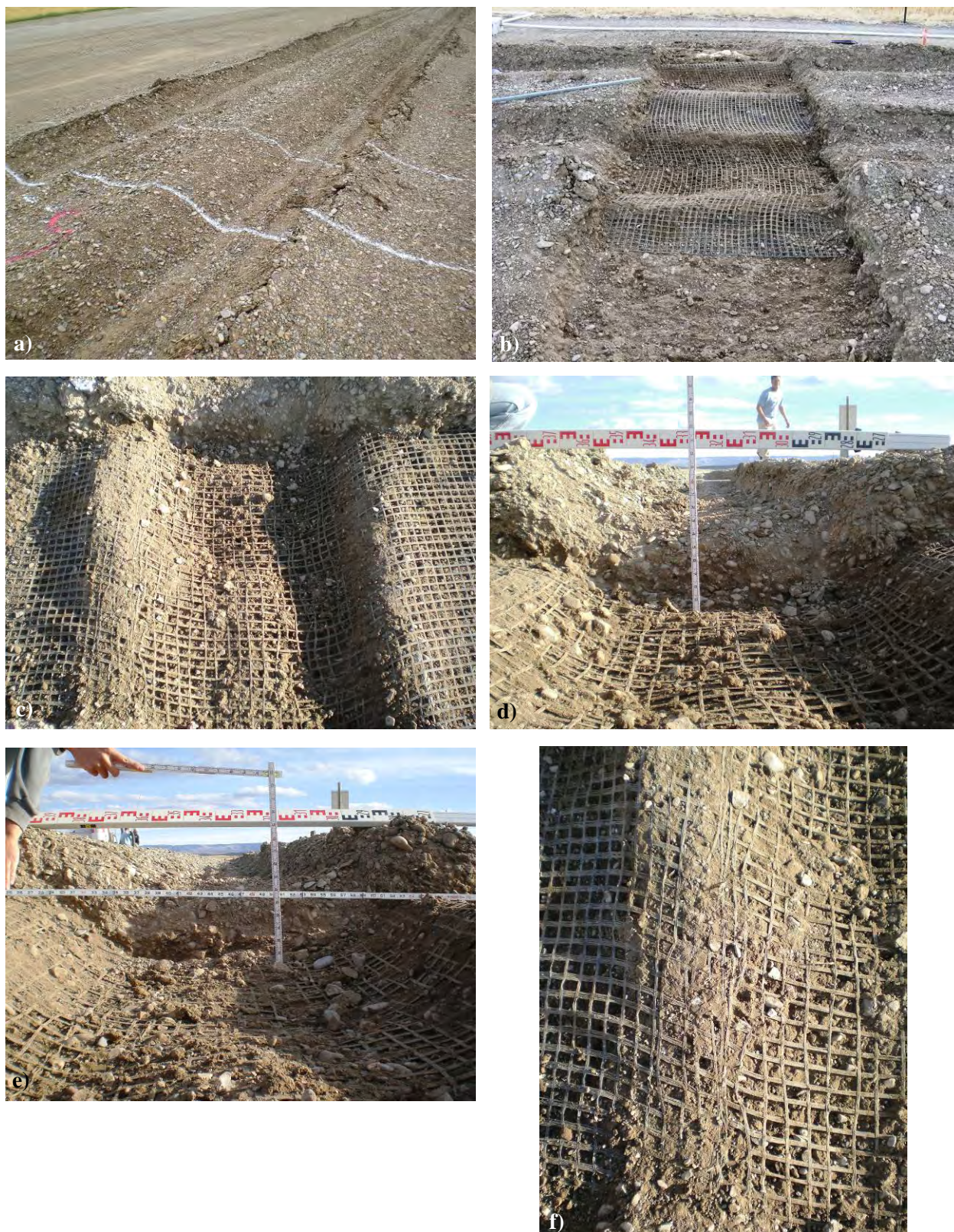
Figure C-28. Photos of the forensic excavations of the WoG-8 test section: a) excavation area, b) looking west, c) rut bowl, d) base rut profile, e) subgrade rut profile and f) close-up of rut.
