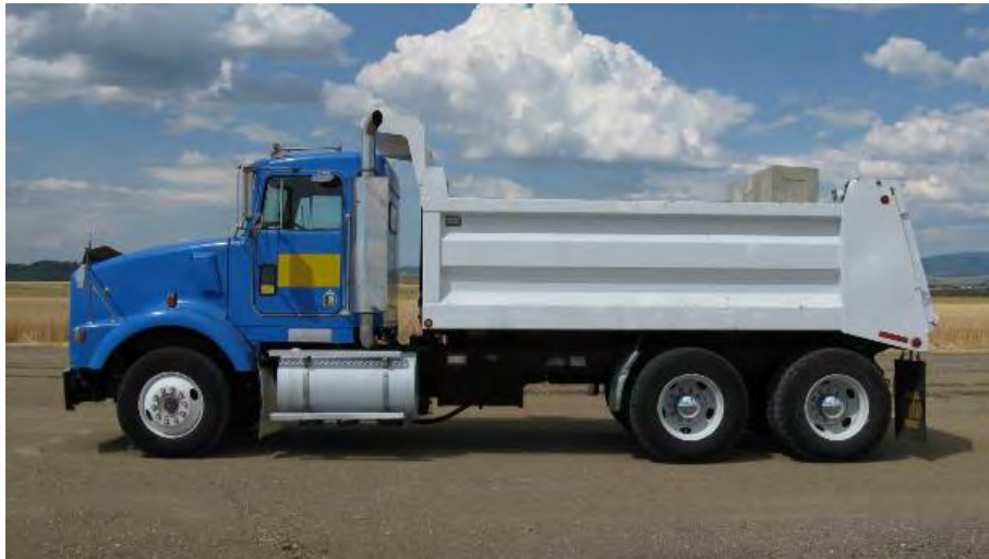
Figure 31. Side view of three-axle dump truck used for trafficking.
