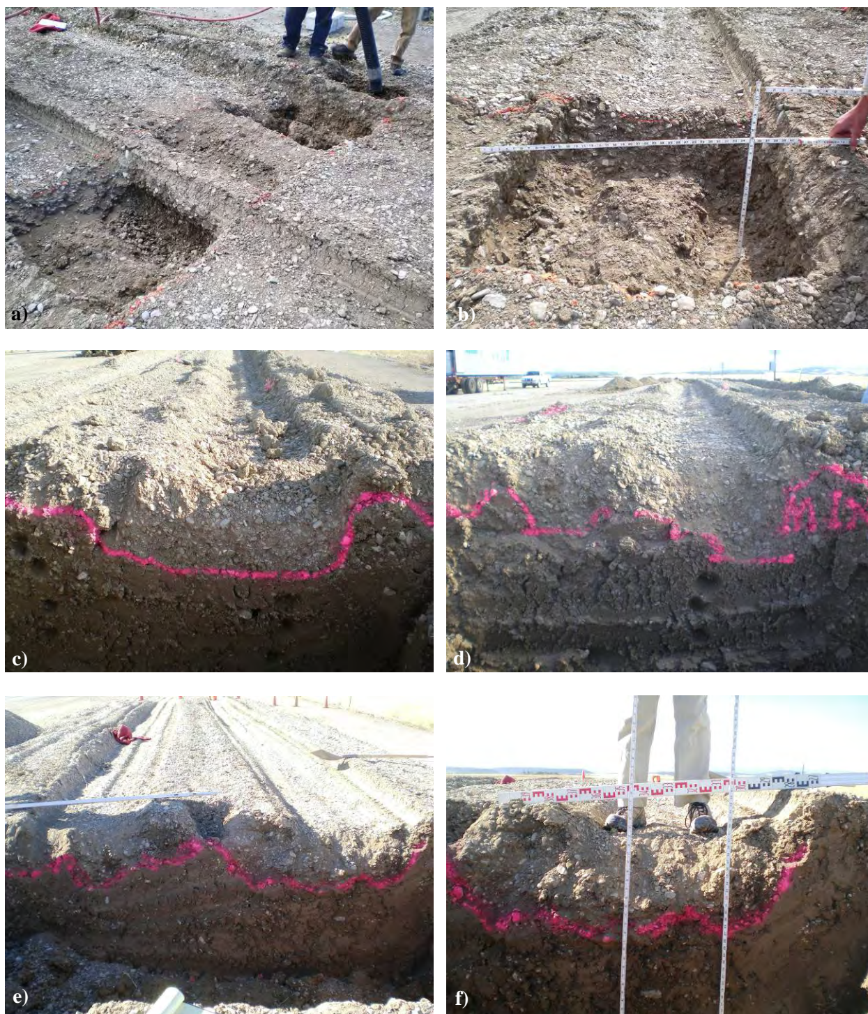
Figure C-5. Photos of the forensic excavations of the Control sections: a) and b) excavation of Control 1, c) and d) rut profile of Control 1, e) and f) rut profile of Control 2.
