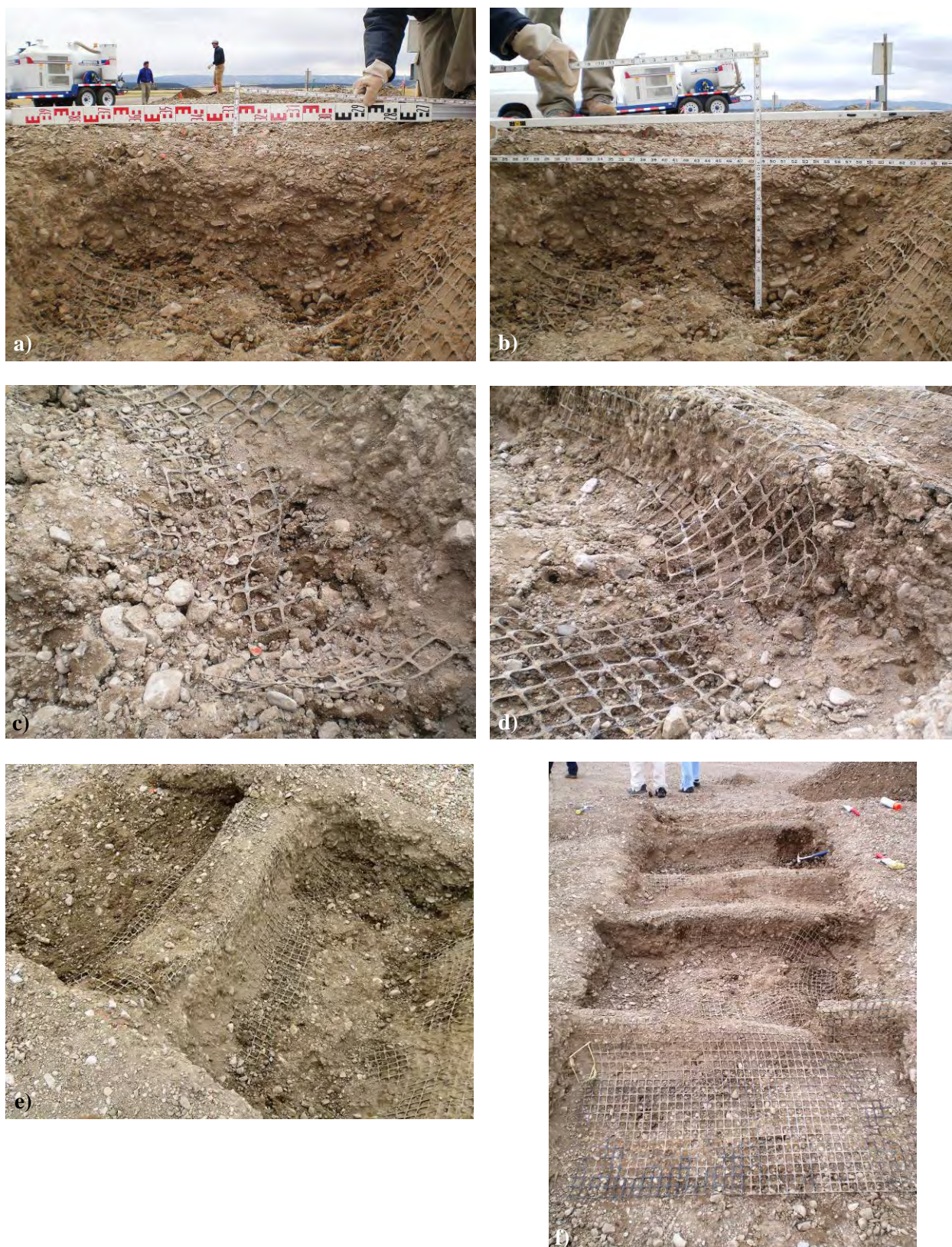
Figure C-19. Photos of the forensic excavations of the IFG-5 test section: a) base rut profile, b) subgrade rut profile, c) close-up of rut, d) close-up of damage, e) rut bowl and f) looking east.
