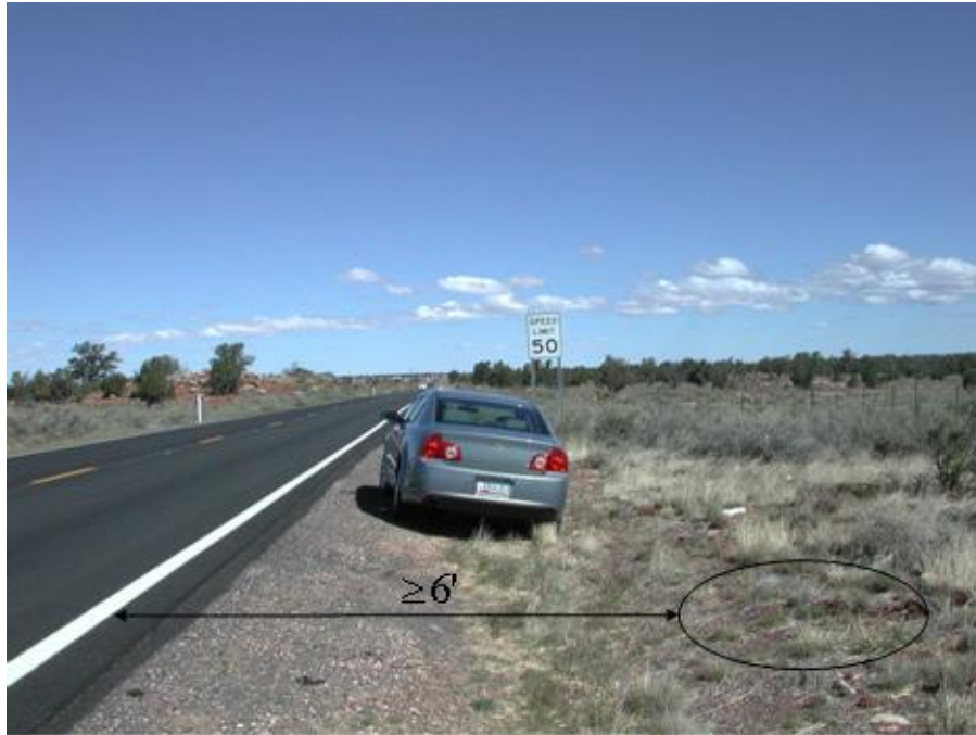
HAR Static Sign Placement on US 180 (Option 2)
