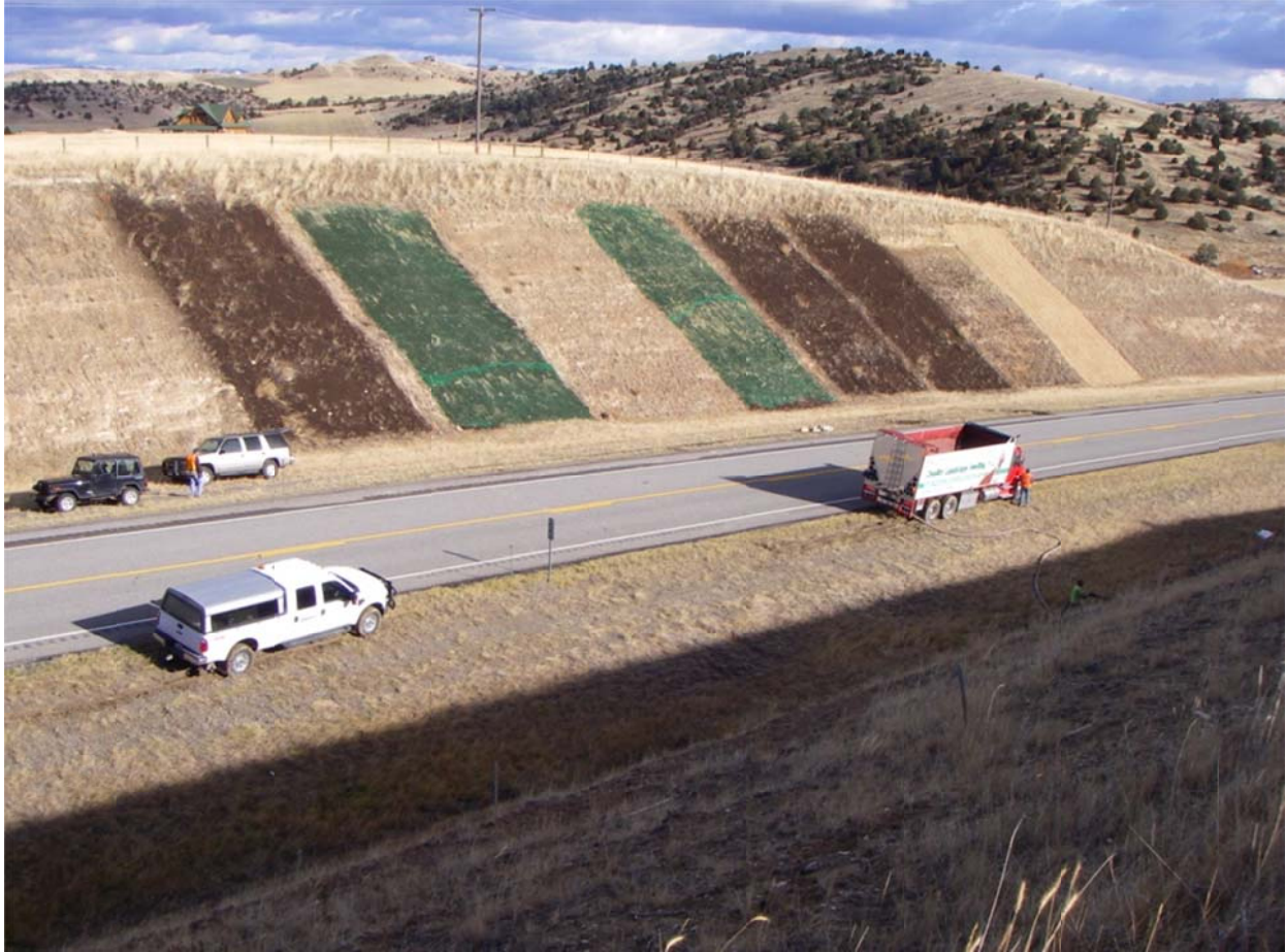
Figure 4: View of eight south-facing plots that are across highway from the four north-facing plots (western plots). Plot 11 is shown furthest to the left in the image (dark colored) while plot 18 is most distant (to the right or east) covered by a tan colored erosion control blanket.
