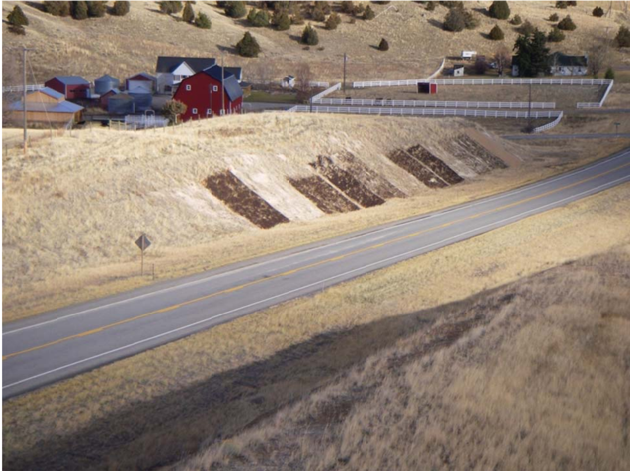
Figure 5: View of 10 south-facing plots that are on the east end of the research site. Plot 1 is furthest to the left in the image (dark colored) and plot 10 is most distant (to the right or east) with a tan colored erosion control blanket.
