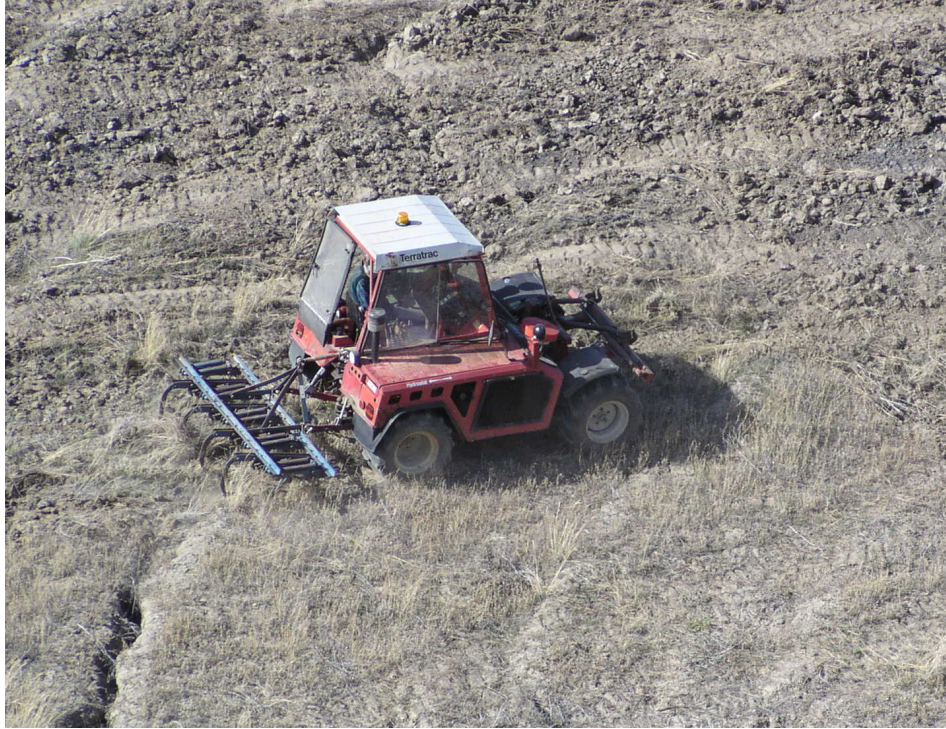
Figure 24. AEBI Terratrak TT88 tilling on the contour along U.S. Highway 12.
