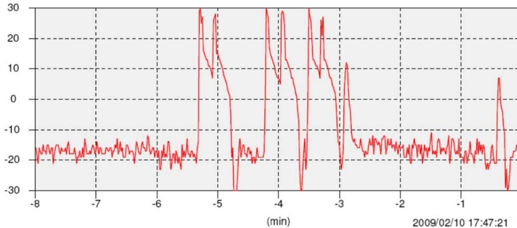
Figure 3.2: Example of a plot generated during reliability testing (x-axis = time; y-axis is signal strength (dB)). In this example, six peaks were identified between 3:00 and 5:30 minutes before the plot was ended. These peaks coincided with a researcher crossing the buried cable at 3 locations (each pass triggered two peaks as the researcher crossed the cable).
