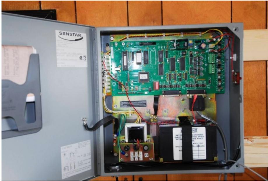
Figure 4.8: The Senstar Perimitrax® Network Controller inside the research trailer (Photo: Marcel Huijser, WTI/MSU).
