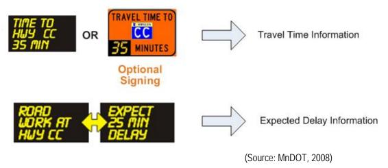
Figure 1 Travel Time and Expected Delay Messages
