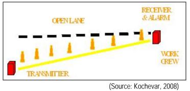
Figure 5 Layout of Safety Line<sup>TM</sup> SL-D12 Work Zone Alarm System
