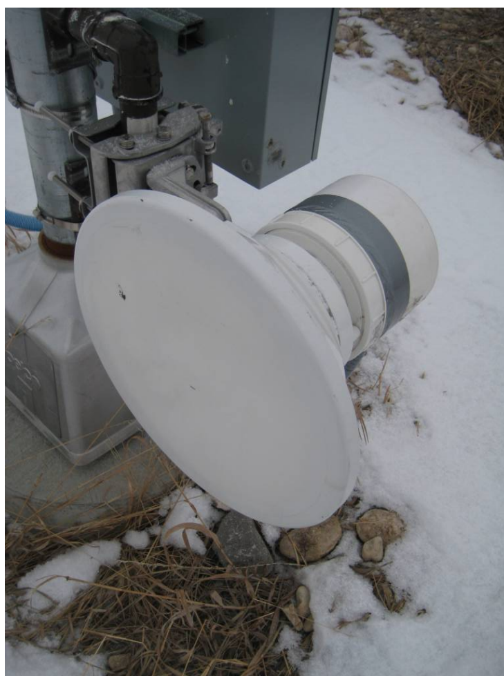
Figure 4.5. The receiver of the third generation break-the-beam system manufactured by ICx Radar Systems. Note: the transmitter looks similar to the receiver.
