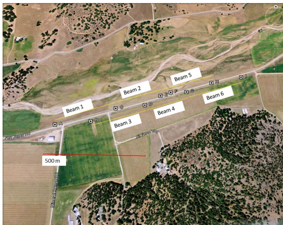
Figure 6.1. Layout of the animal detection system along SR 3 near Ft Jones, CA. Letters indicate poles, numbers and yellow lines indicate beams.
