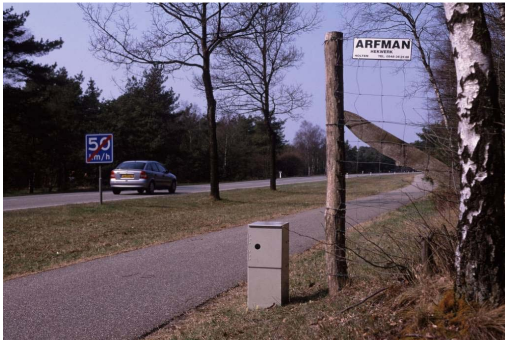
Figure 46. An animal detection system (infrared break-the-beam system manufactured by Calonder Energy, Switzerland) at a gap in a wildlife fence near ‘t Harde, The Netherlands (© Marcel Huijser).
