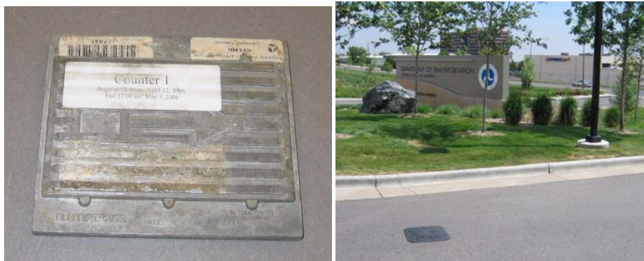
Figure 1: Traffic Counter (left) and Traffic Counter Deployed (right) i
