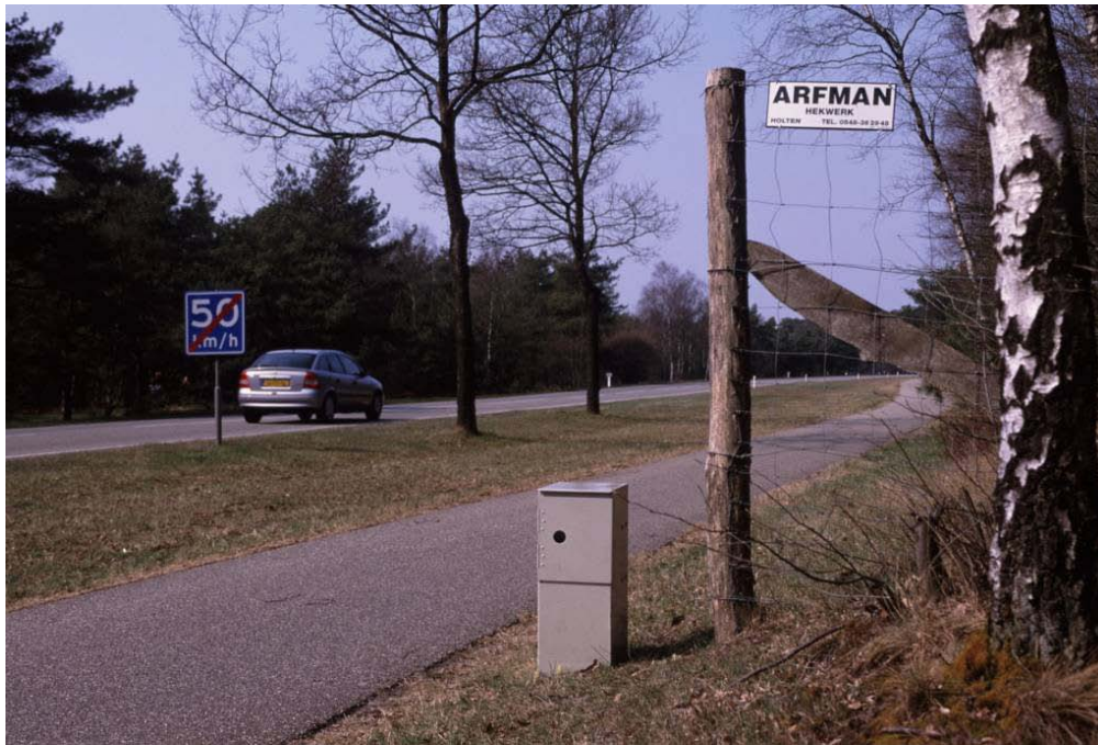
Figure 49. An animal detection system (infrared break-the-beam system manufactured by Calonder Energy, Switzerland) at a gap in a wildlife fence near 't Harde, The Netherlands (© Marcel Huijser).
