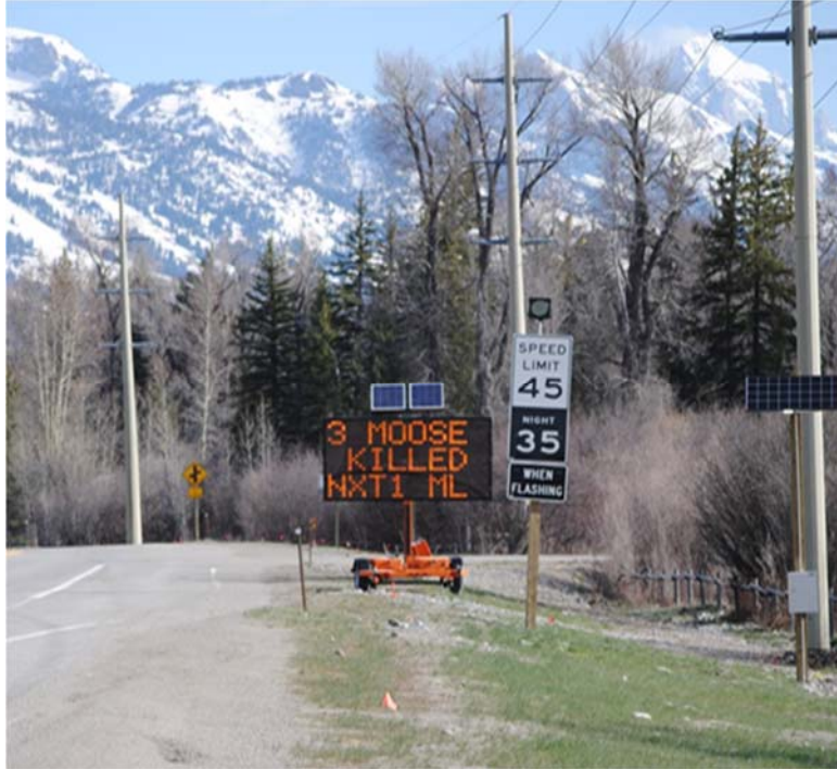
Figure 8-4 Dynamic Message Sign on WY Highway 390 (Photo credit: Rob Ament/WTI)
