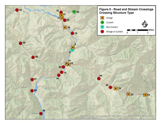
Figure 28. Zoomed in overview of the stream crossings in a part Teton County (see Figure 24 for overview).
