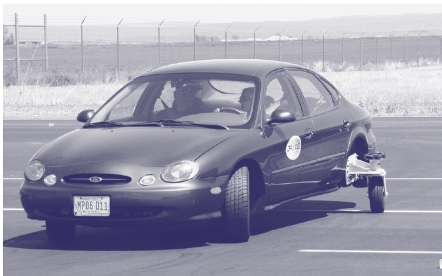
The Skid Monster™ enables a driving instructor to simulate skid conditions while travelling at lower speeds and without altering the driving surface.
