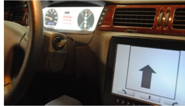
Example of two visual displays from different driver support systems (brake warning, navigation).
