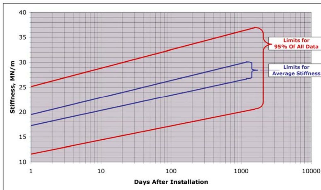
Figure 3 Acceptable Stiffness Limits Soil~Sement Amended ASSHTO A-2 Silty Sand
