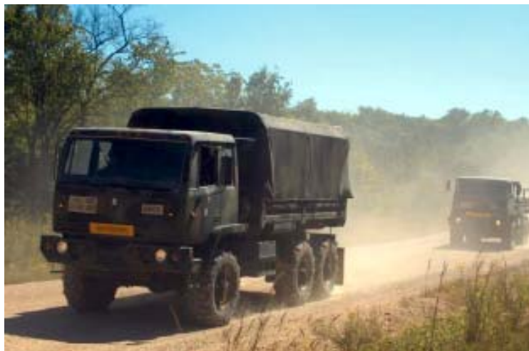
Figure 4. Dust generation caused by military convoys operating on unpaved road.
