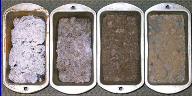
Dust control application of 30 percent MgCl 2 solution Samples oven dried 48 hours
