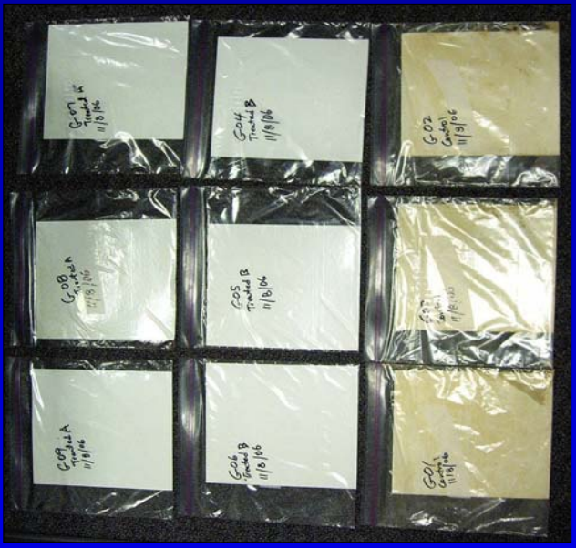
Dust control application of 30 percent MgCl 2 solution Samples oven dried 48 hours
