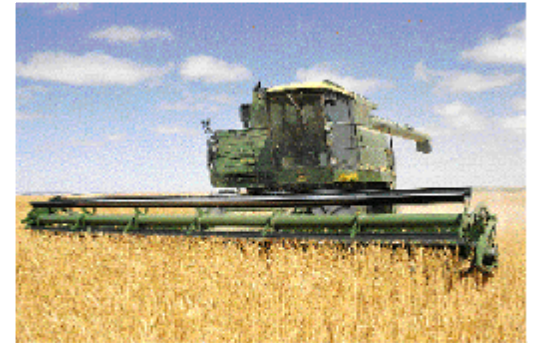
This grain combine can be outfitted with a GPS receiver, yield monitor, and electronic sensors to track crop production based on location. These data can be transferred to a geographic information system to create a yield map and subsequently used to analyze the field and make site-specific management decisions.
