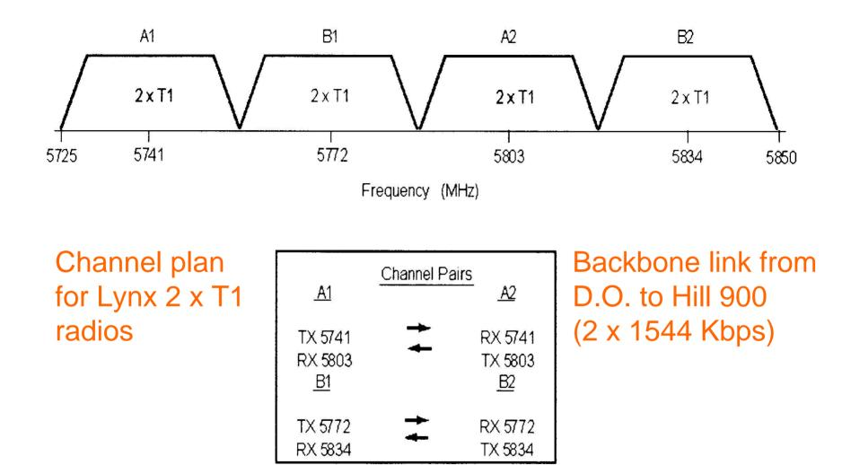
Figure 3-4: Channel Plan, 5.8 GHz 2xT1
