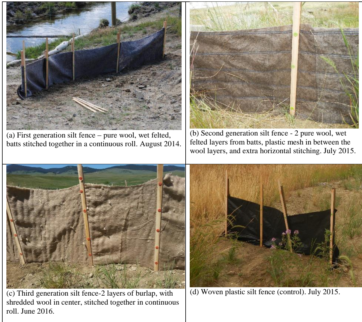
Figure 2. Three generations of wool silt fence and the standard woven plastic silt fence tested in field trials, 2014 – 2016.
