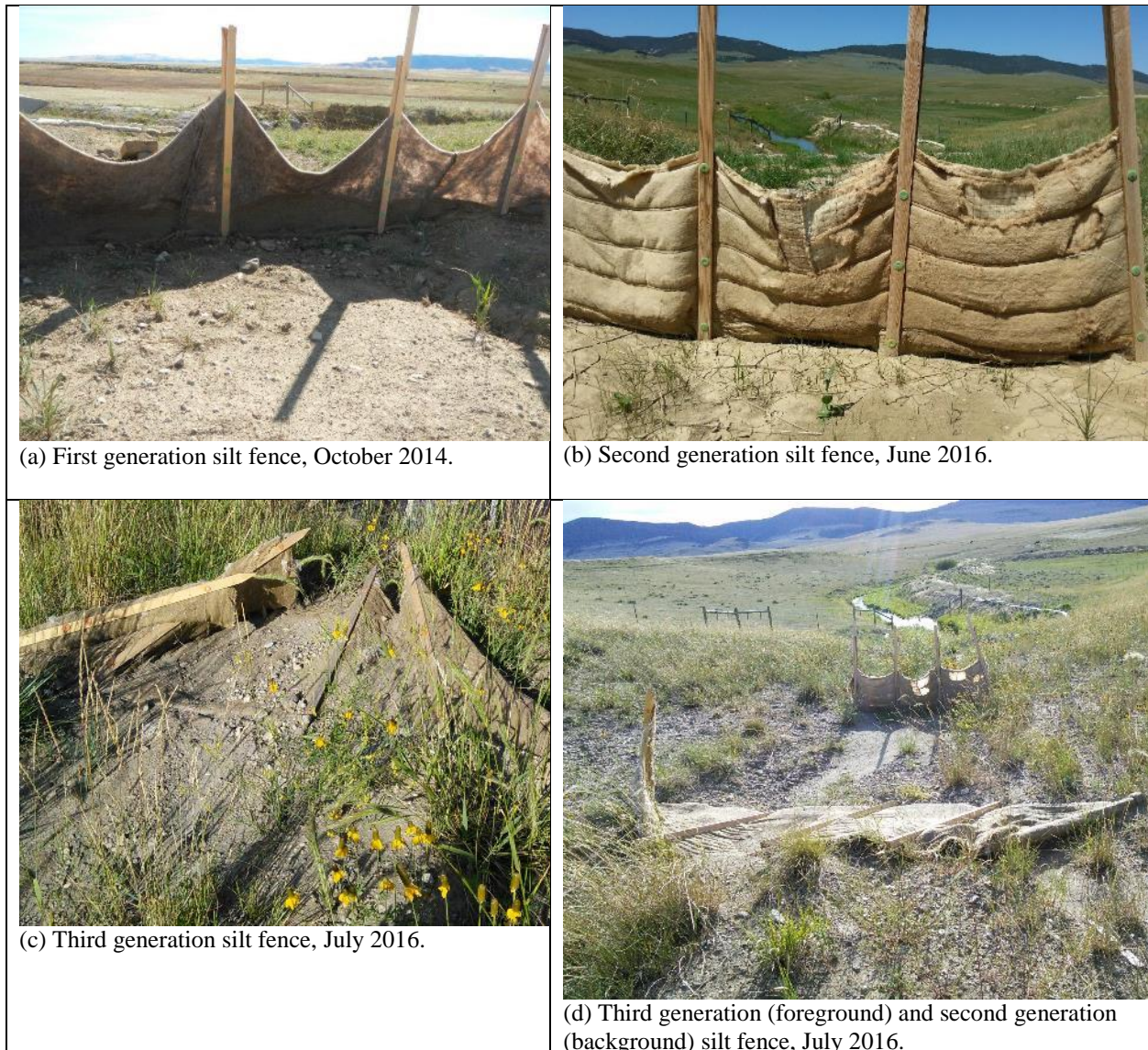
Figure 6. Photo monitoring the three generations of wool silt fence developed and tested in field trials along U.S. Highway 12, 2014 – 2016.
