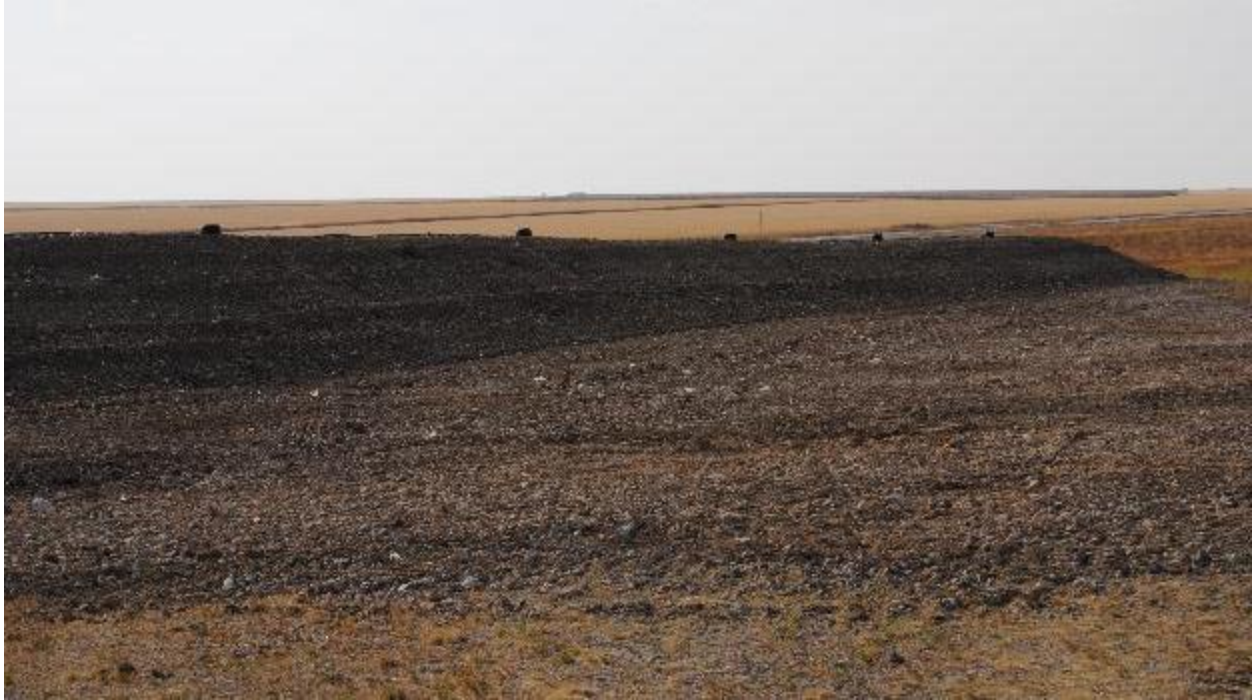
Figure 4. Test slope (2H:1V) constructed at Transcend, a WTI-MSU experimental station in Lewistown, MT.
