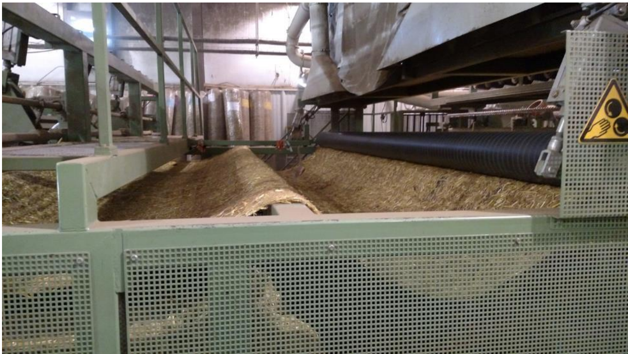
Figure 5: Close up of a straw and jute net ECB manufacturing at Ero-Guard, Mapleton, MN.
