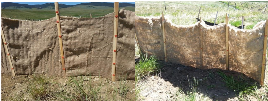
Figure 6 (a): Rolled silt fence constructed of two burlap layers sewn together with cut wool pieces as filler. (b) Backlit burlap and wool silt fence shows the lack of consistency in the distribution of the wool pieces in the center layer of the fence.
