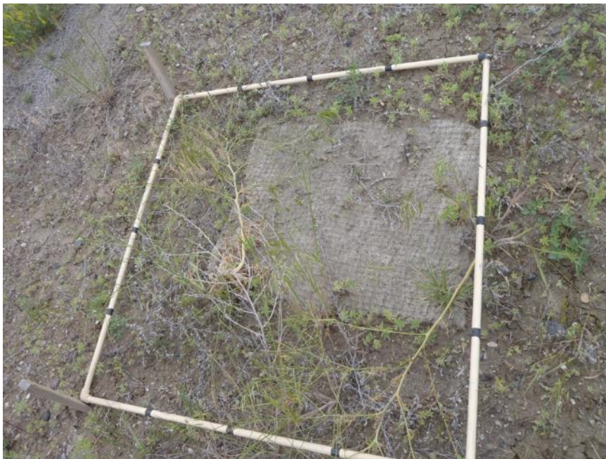
Figure 2: June 2016 field monitoring found shrinkage of a pure wool needle punched batt along US Hwy 287 near Three Forks, MT. The product initially covered the entire one square meter within the PVC frame.
