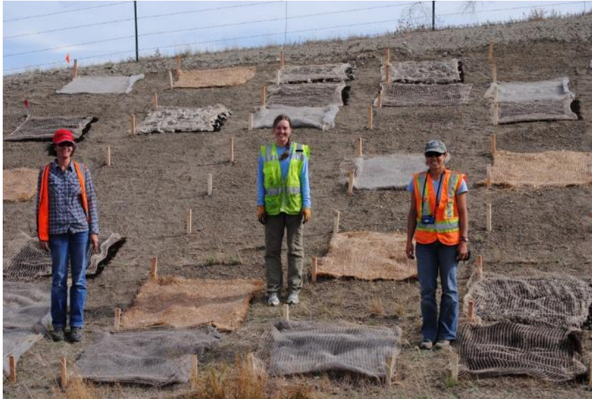
Figure 1. Replications of erosion control products along US Hwy 287, Three Forks, Montana, October 2014. Plot dimension is one meter square and all treatments are covered with mesh netting stapled in place.
