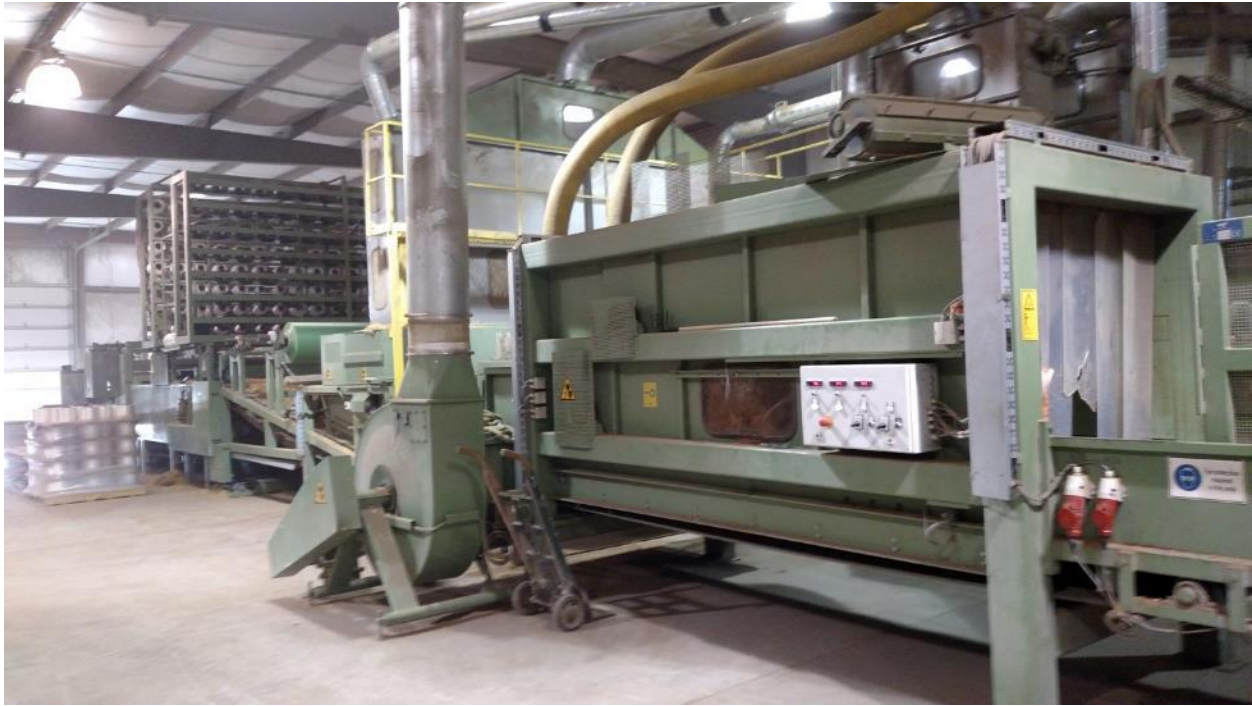
Figure 4: Equipment that manufactures rolled ECBs, Ero-Guard, Mapleton, MN.
