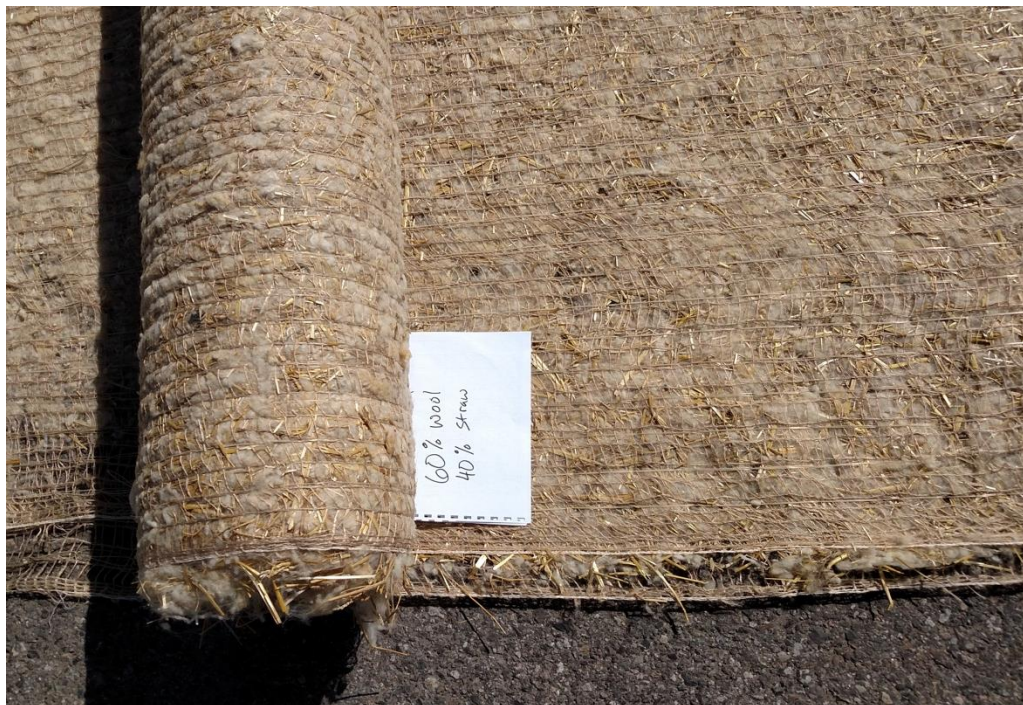
Figure 3. Example of wool combined with straw as fill between two biodegradable net layers in a rolled ECB.
