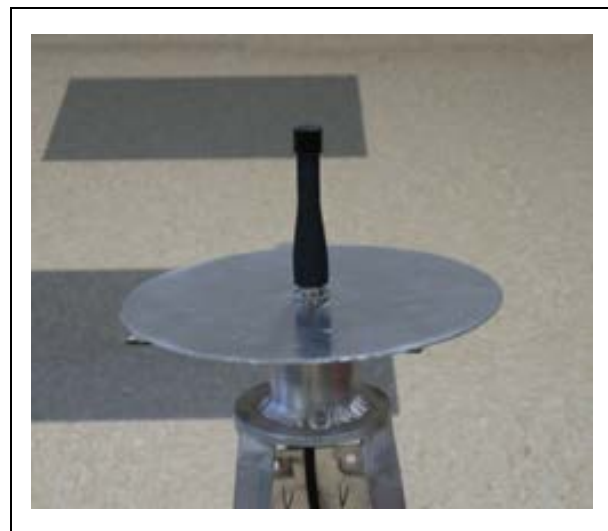
Figure 27: Small Ground Plane - WTI Photo
