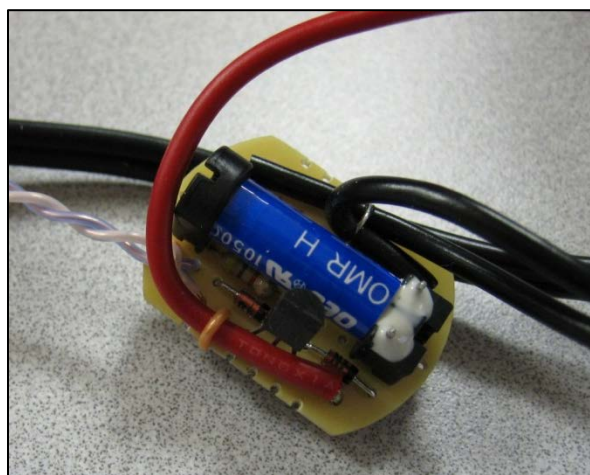
Figure 10: Prototype Light Switch – WTI Photo
