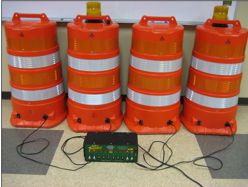
Figure 38: sDrum Charging – WTI Photo
