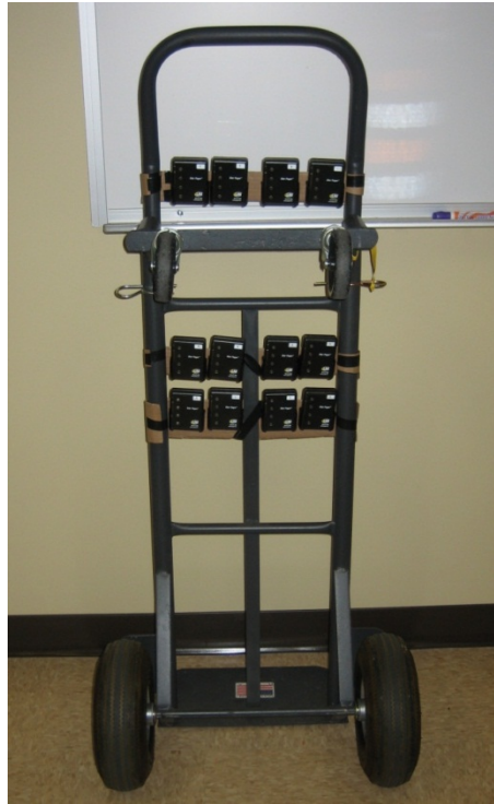
Figure 25: Pager Range Test Fixture - WTI Photo
