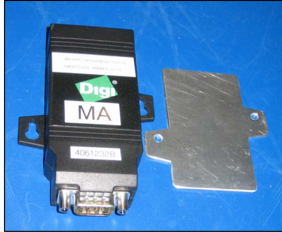
Figure 39: Digi Radio with Mounting Plate – WTI Photo
