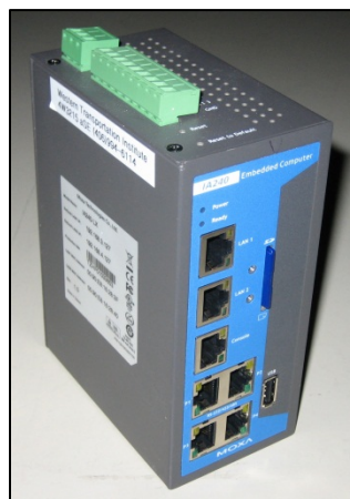
Figure 5: Moxa Model IA240-LX Industrial Computer – WTI Photo
