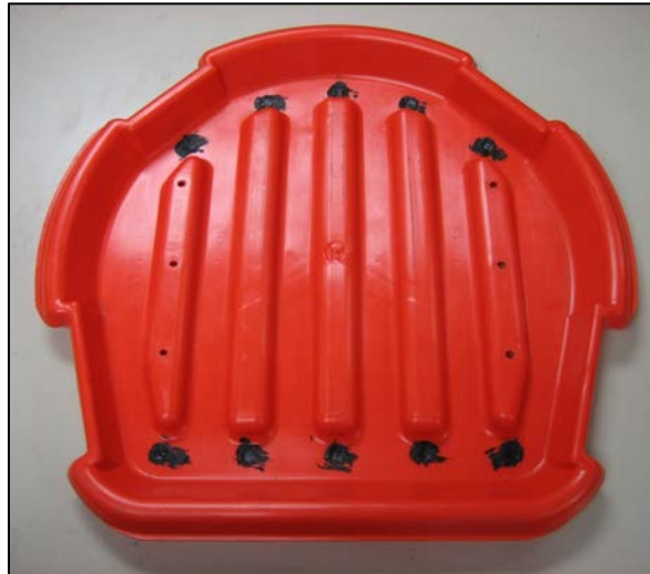
Figure 34: Traffic Standard Drum Base with Tabs Removed - WTI Photo
