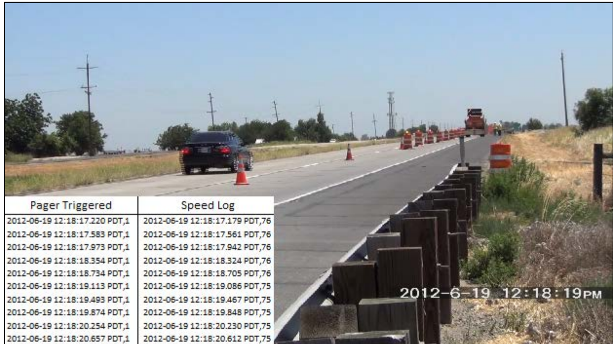
Figure 65: Frame Capture of Speeding Vehicle - WTI Image
