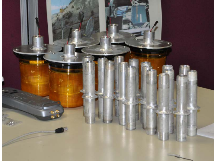
Figure 14: Light Mounting Plate and Light Pipe – WTI Photo
