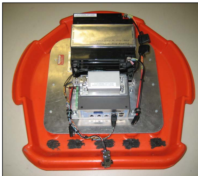
Figure 44: Master/Logger sDrum Base Assembly – WTI Photo
