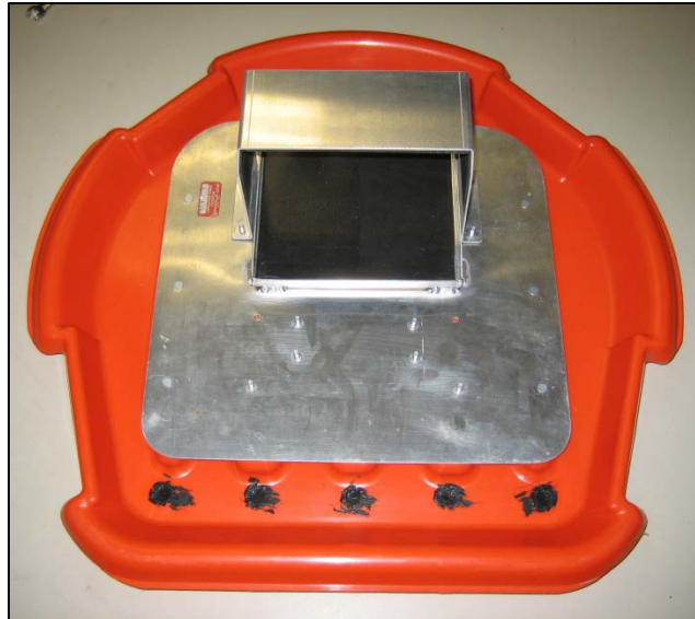
Figure 43: Battery Tray and Strap – WTI Photo
