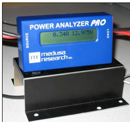
Figure 18: Power Analyzer Pro – WTI Photo
