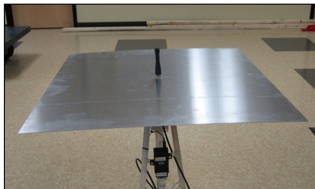
Figure 28: Large Ground Plane - WTI Photo
