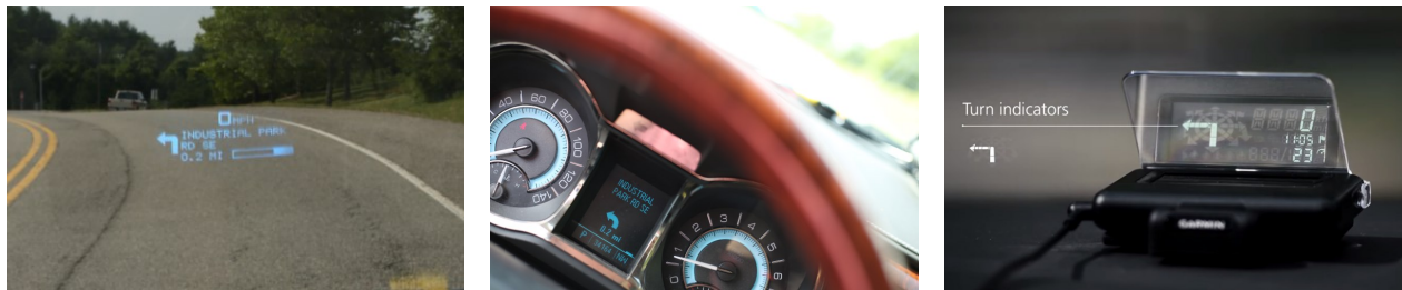
Figure 4. Left: 2010 Buick Lacrosse HUD. Center: 2010 Buick Lacrosse HDD. Right: Garmin Navigational HUD.
