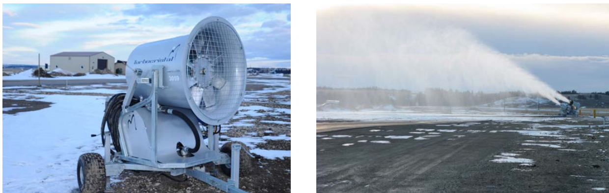
Figure 3: Fan gun snowmaker (left), man-made snow event across the test track (right).
