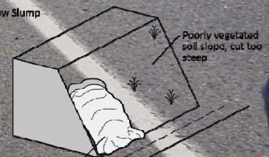
Shallow, flow-type failure in soil
