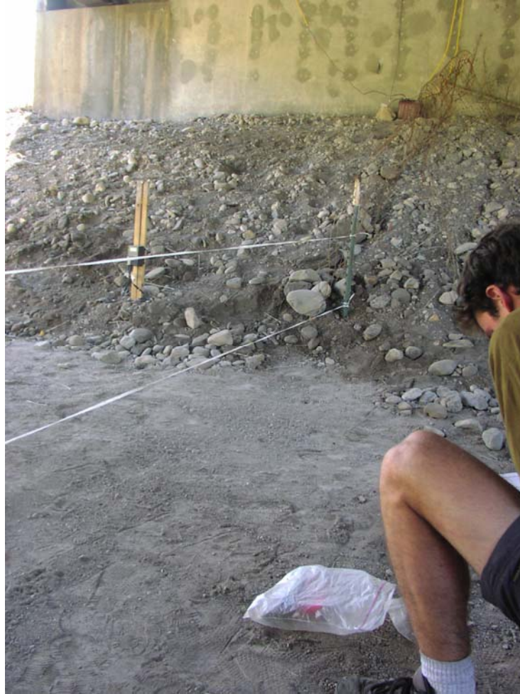
Photo 5. Two-strand system of barbed-wire/sticky string used to snag DNA/hair sample of individual animals using wildlife underpass.
