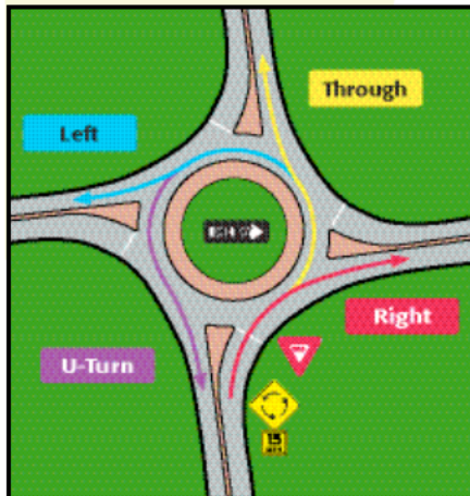
Figure 3. Roundabout Signage and Traffic Flow
