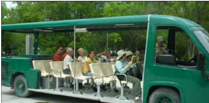
The current tram engine unit includes passenger seating and can operate alone or with trailers.
