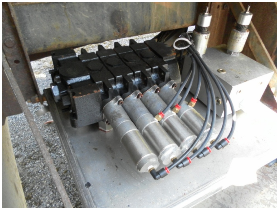
Figure 38. Hydraulic components showing little to no corrosion due to sealed protective cover.
