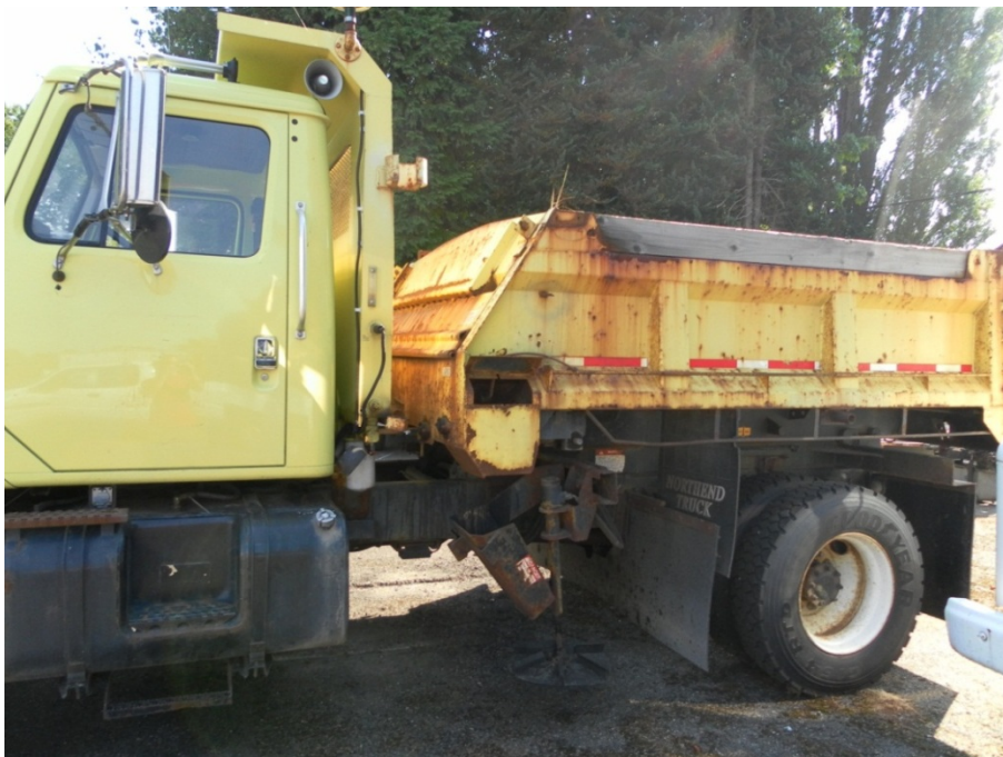
Figure 36. Side discharge salt spreader showing extensive corrosion.
