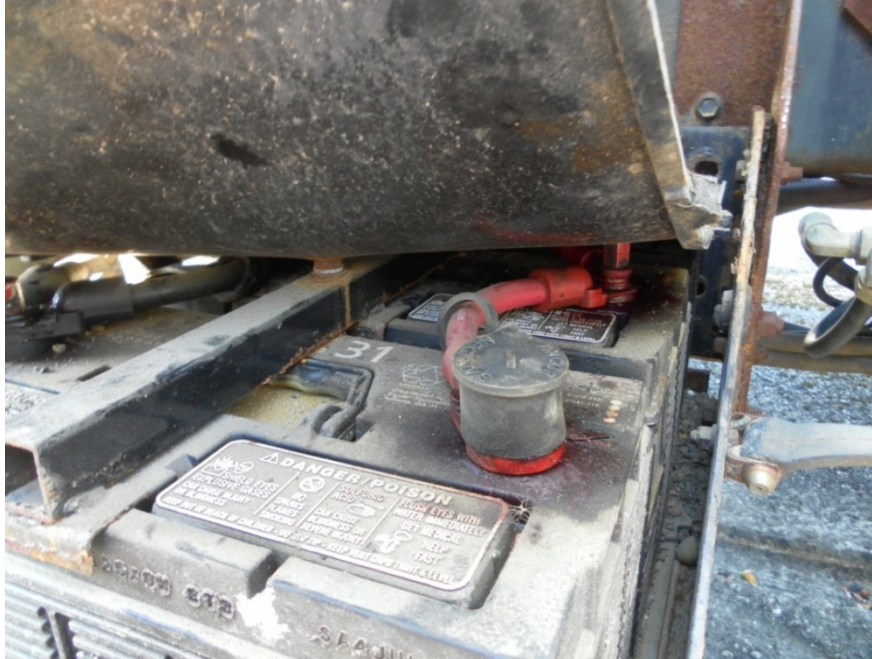
Figure 41. Rubber caps on battery terminals used to mitigate effects of corrosion.
