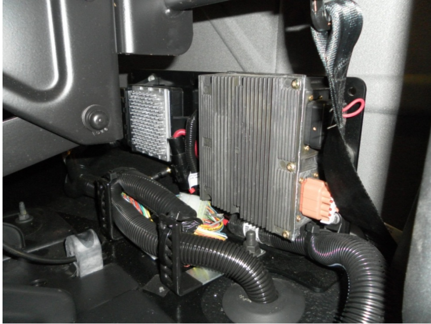
Figure 43. Modified electrical junction boxes are mounted inside the cab off the floor.
