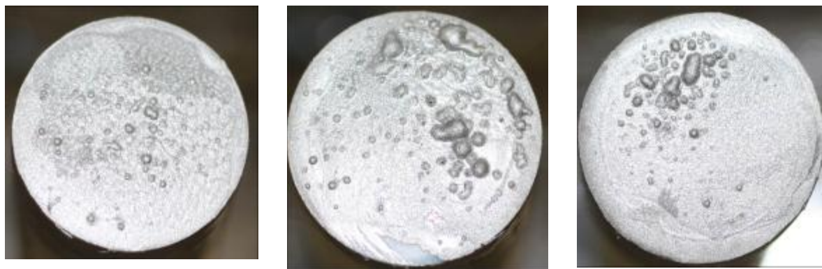
Figure 26. Sensor surface morphology after 8 cyclic exposure in 3.0% \text{MgCl}_2 deicer environment: (a) control group, (b) sensors spray-applied with inhibitor Krown T40 , (c) sensors spray-applied with inhibitor Rust Oleum , and (d) sensors protected by coating Rust Bullet . Sensor material: Left: 1100 Al; Middle: 304 SS; Right: 1008 CS
