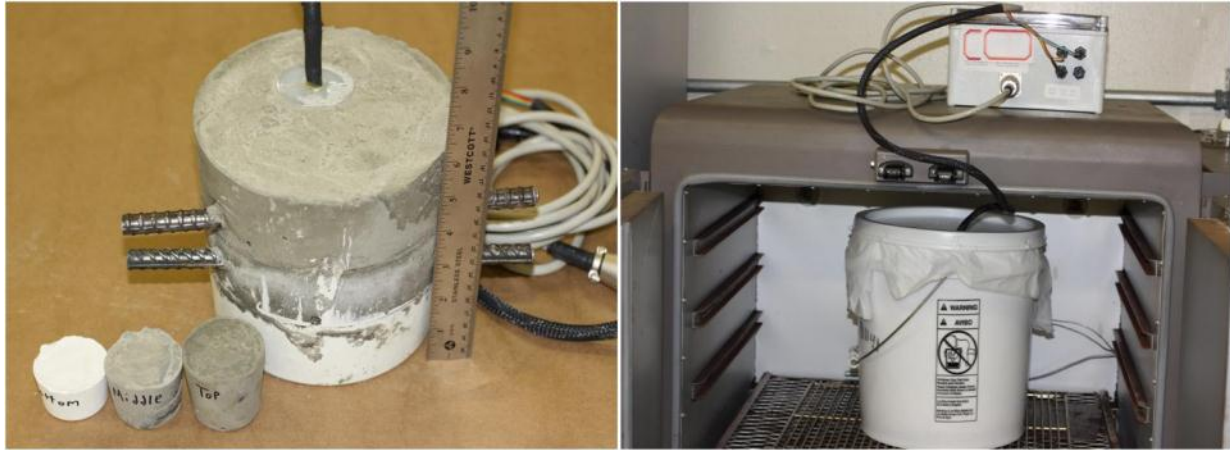
Figure 15. Photographic illustration of the fabrication and curing procedures of paste specimen with multi-probe sensor embedded. (a) Positioning mold and the sensor; (b) Pouring the bottom paste layer(2 ½" thickness); (c) Preparing the middle paste layer after 24 hours of bottom paste layer pouring (with a 6" length #5 rebar inserted into the mold); (d) Pouring the middle paste layer(1 ½" thickness); (e) Preparing the top paste layer after 24 hours of bottom paste layer pouring (with a 6" length #5 rebar inserted into the mold); (f) Pouring the top paste layer(2" thickness); (g) de-mold the paste specimen after 24 hours of top paste layer pouring (a small paste cylinder of each layer paste shown was fabricated for further chloride and pH analysis); (h) Placing the specimen in a humidity chamber for 28 days curing process.
