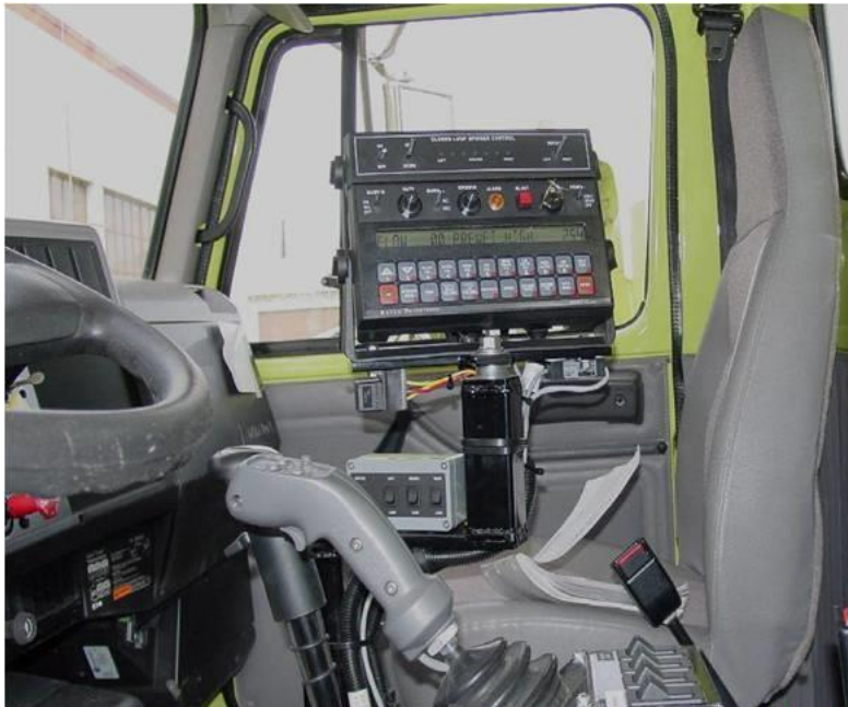
Figure 3-4: Open and closed loop controllers maintain a constant material application rates (Washington State Department of Transportation photo)
