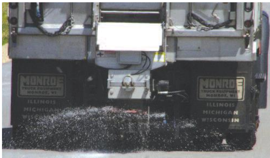
Figure 3-7: Salt slurry generator in operation (Monroe Truck Equipment Inc. photo)
