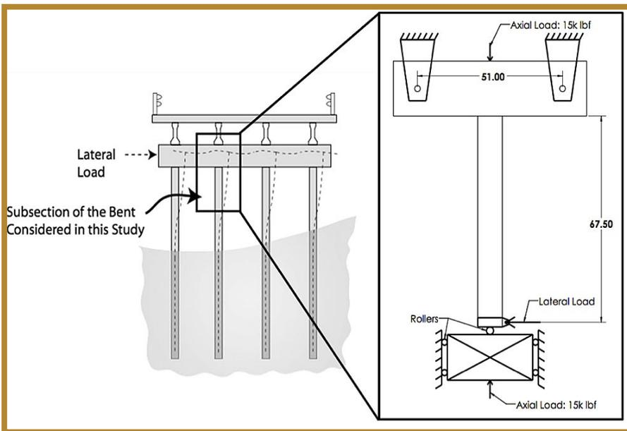
Figure 2 - General Test Setup
