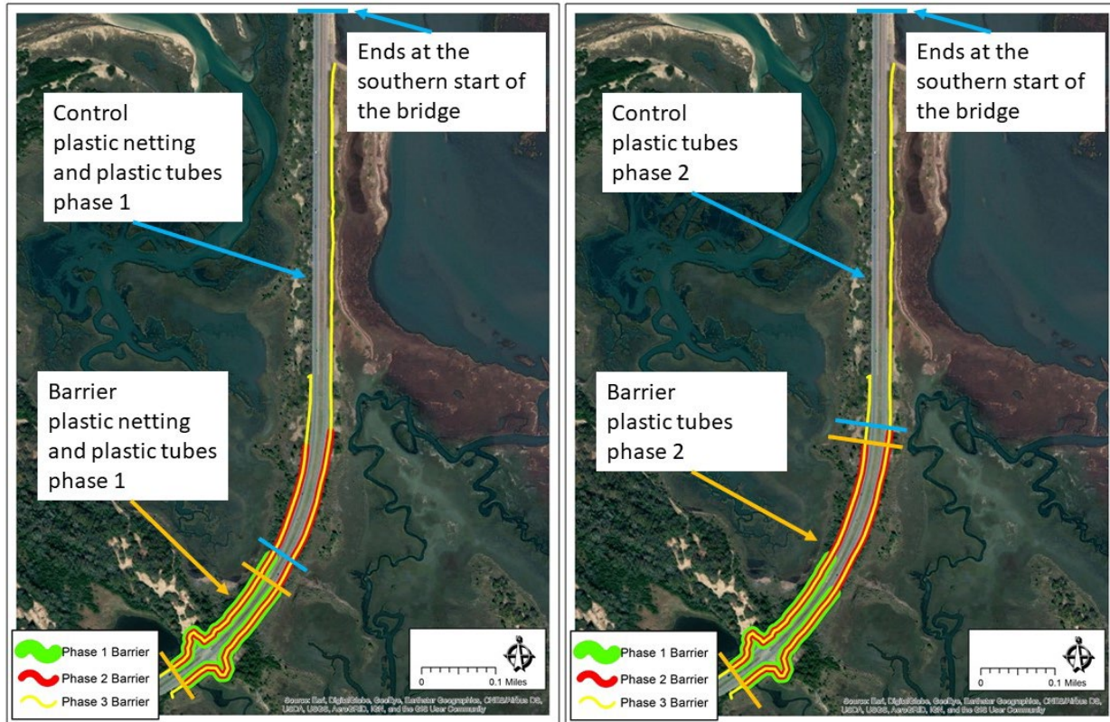
Figure 14: The Treatment (Barrier) sections) and the Control sections for the BACI analyses for phase 1 (left) and phase 2 (right). Note: The South end treatment (barrier) coincides with the start of the barrier of phase 1/2, north end control coincides with the start of the bridge.
