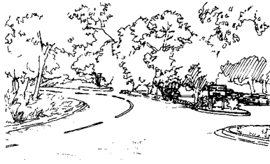
An example of a visitor center turnout that is clearly marked and signed, and separated from the road with a bermed island featuring indigenous plant material.
