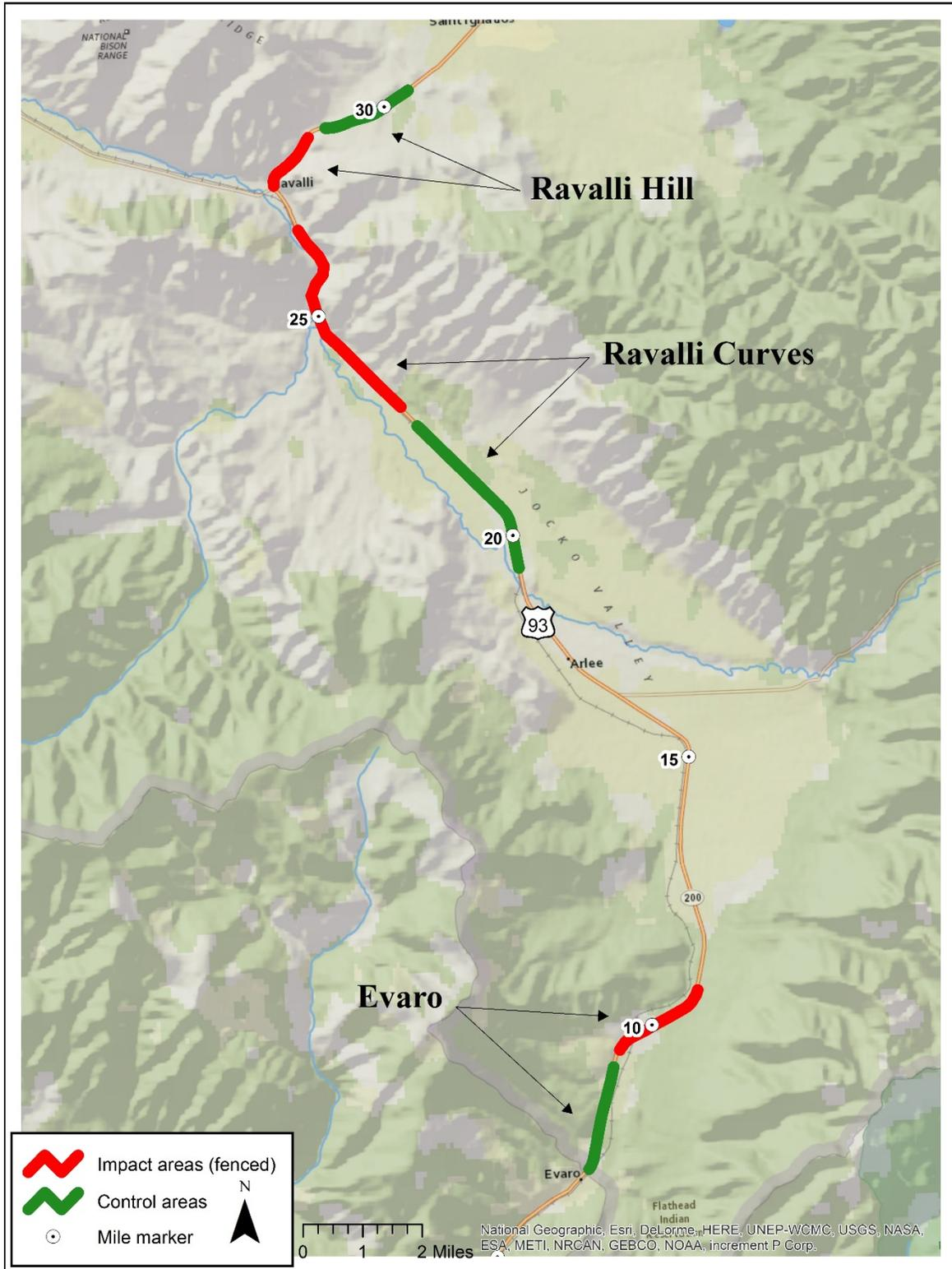
**Figure 3: Impact road sections with wildlife fences (in red) and control road sections without wildlife fences (in green) in the Evaro, Ravalli Curves and Ravalli Hill areas.**
