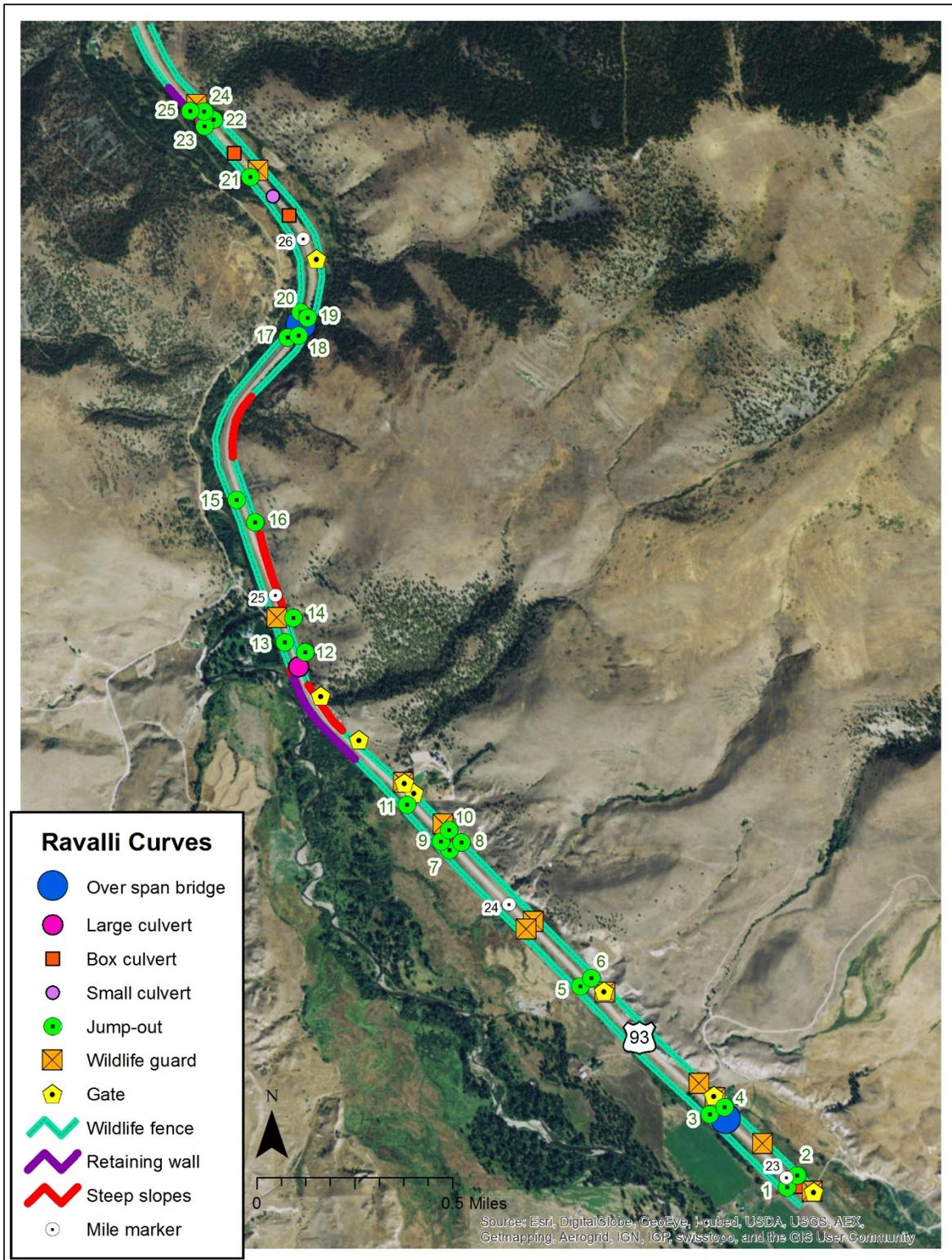
Figure 35: The jump-outs and other mitigation measures in the Ravalli Curves area.
