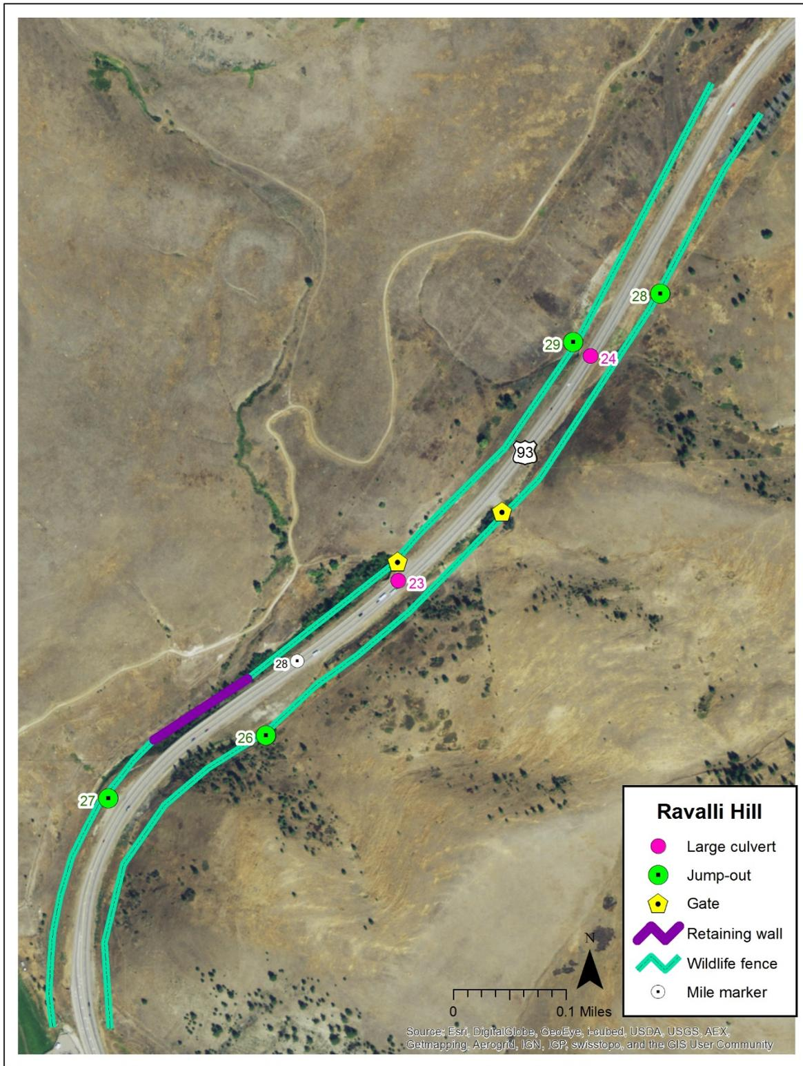
Figure 36: The jump-outs and other mitigation measures in the Ravalli Hill area.
